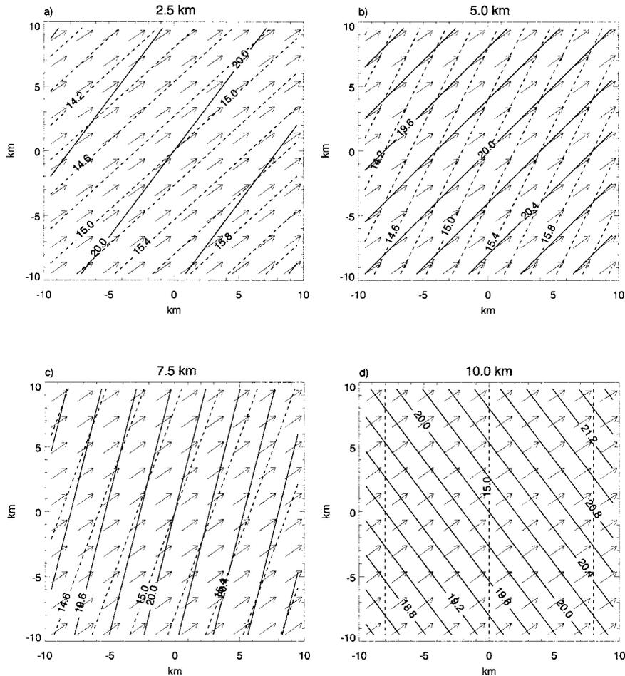
FIG. 1. Linear wind used in section 3. Full lines are isolines of the  $u$  component and dashed lines of the  $v$  component of the horizontal wind field. Contours are drawn each  $0.2 \text{ m s}^{-1}$ . Arrows indicate the full horizontal wind vectors.
