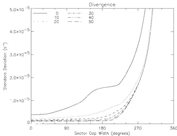
FIG. 6. Standard deviation of estimated divergence of the highest model level as a function of increasing sector gap for various assimilation periods. The amplitude of true divergence is  $5 \times 10^{-5} \text{ s}^{-1}$ .
