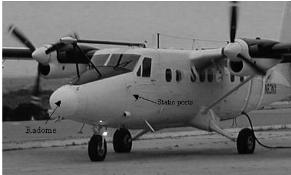
FIG. 1. Photograph of the CIRPAS Twin Otter showing the arrangement of the radome, the static pressure ports (starboard side), and the wind-propeller system.
