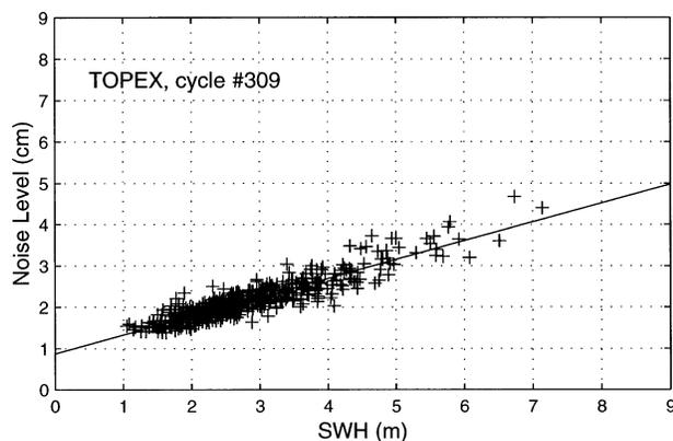
FIG. 5. TOPEX rms white-noise-level estimates with respect to SWH based on 5-min track segments of cycle 309.
