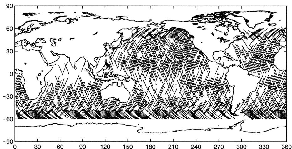
FIG. 1. Spatial distribution of the 5-min track segments used to assess the noise-level estimates for cycle 7 of GFO.
