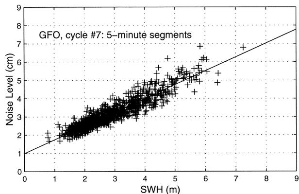
FIG. 2. GFO rms white-noise-level estimates with respect to SWH based on 5-min track segments of cycle 7 of GFO.
