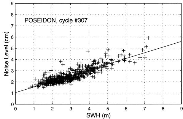
FIG. 7. Poseidon rms white-noise-level estimates with respect to SWH based on 5-min track segments of cycle 307.
