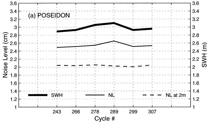
FIG. 8. Variation of the average value of NL and SWH for each Poseidon cycle (note the time discontinuities), based on 5-min segments, along with the value of NL at 2-m SWH, determined from the linear fit, as a function of the cycle number.
