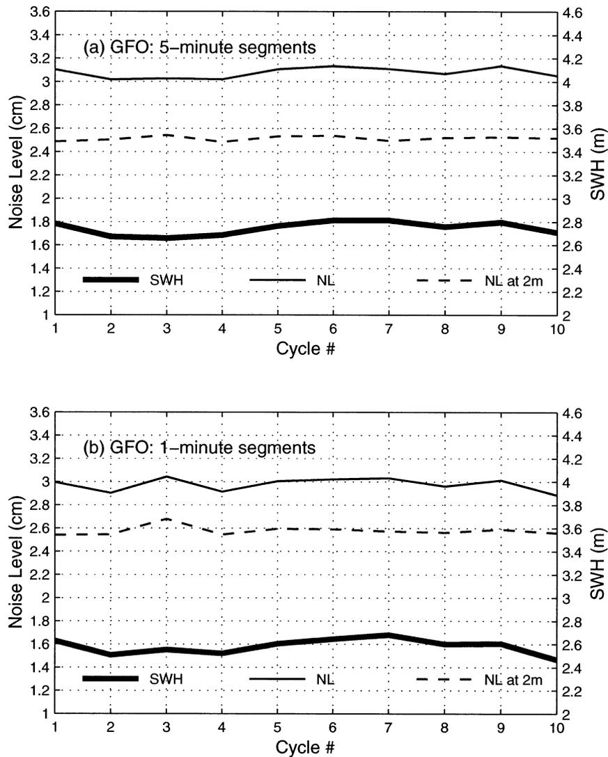
FIG. 4. Variation of the average value of the noise level (NL) and SWH for each GFO cycle, along with the value of the noise level at 2-m SWH, determined from the linear fit, as a function of the cycle number: (a) results for the 5-min segments and (b) results for the 1-min segments.
