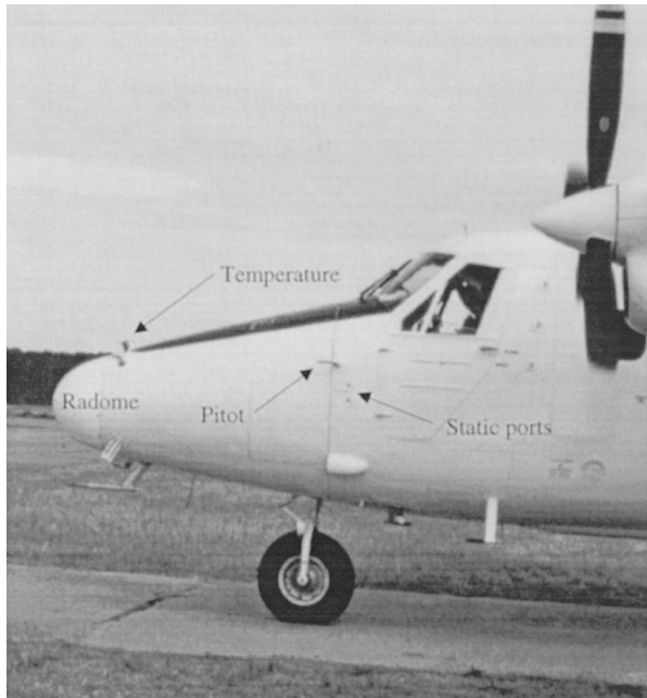
FIG. 1. Photograph of the CIRPAS Twin Otter showing the various probes near the aircraft nose.
