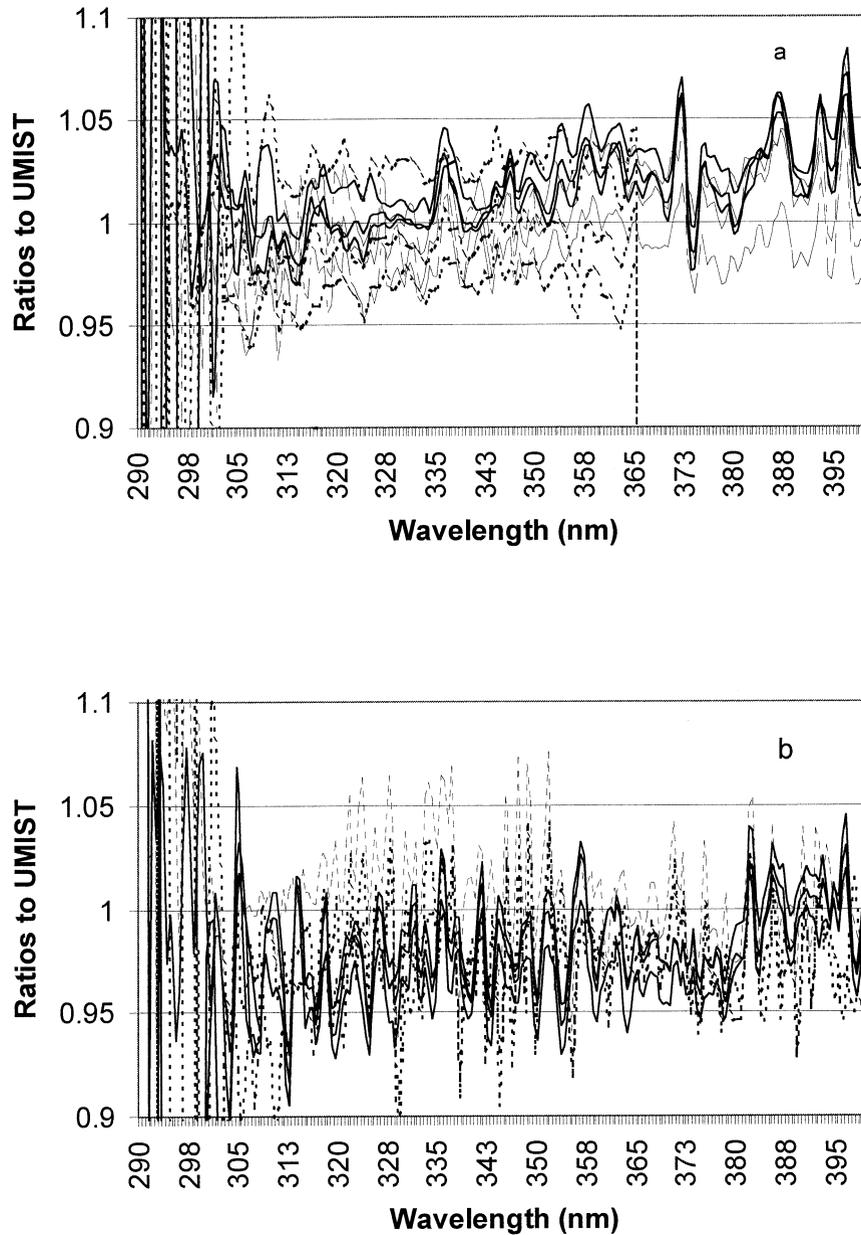
FIG. 2. Results of the three stability checks on day 222 expressed as a ratio of each instrument to the UMIST measurement for (a) global irradiance at SZA of  $71^\circ$ ,  $24^\circ$ , and  $64^\circ$  (UIIMP, solid lines; AUTH, dotted lines; IFU, dashed lines) and (b) actinic flux at SZA of  $66^\circ$ ,  $24^\circ$ , and  $70^\circ$  (IFU, solid lines; METCON, dotted lines).
