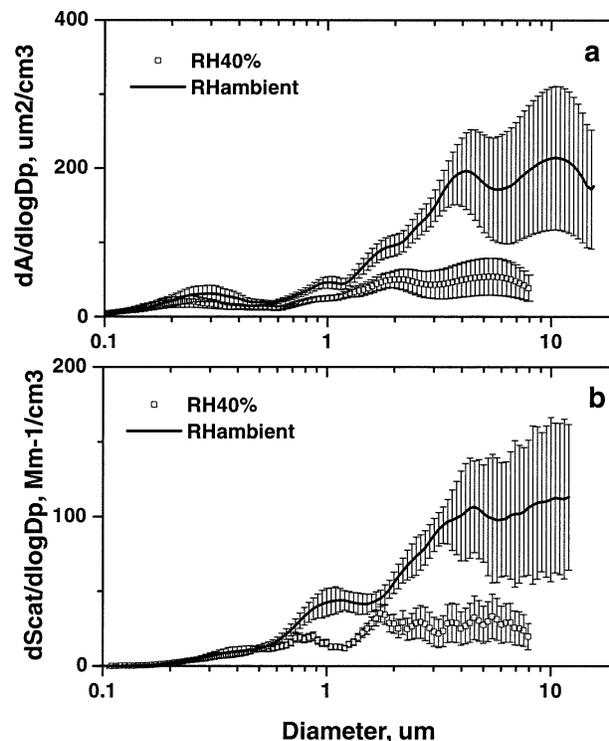
FIG. 7. Comparison of (a) surface area and (b) calculated scattering distributions over size for both dry 40% RH and ambient humidity conditions during the first half of the SEAS experiment.
