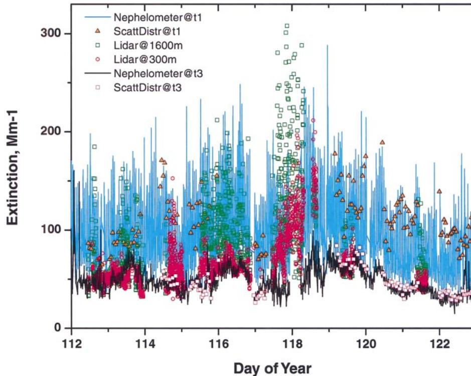
FIG. 10. Time series of 5-m (t1) continuous extinction data (blue lines) and 20-m (t3) extinction data (black lines) corrected to ambient conditions. Corresponding extinction calculated with 20-min averages from size distribution at t1 (triangles) and t3 (red open boxes) compared to variations in lidar extinction observed 300 m offshore from 0–25 m (circles) and at 1600 m offshore near the reef (green open boxes).
