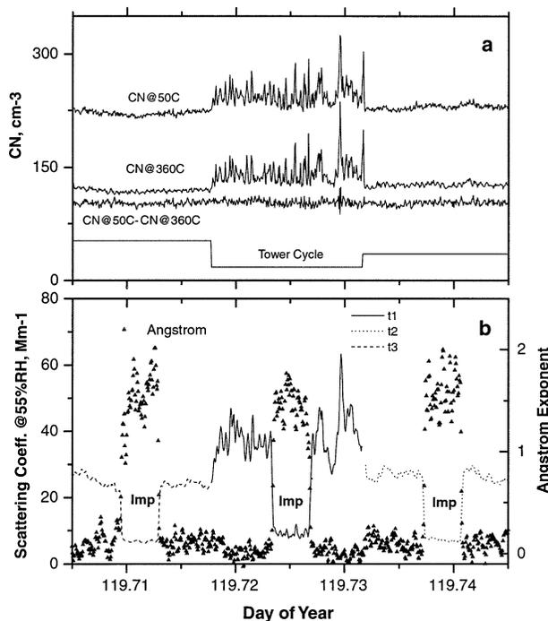
FIG. 3. A 1-h time series showing (a) CN at 50° and 360°C and their difference and (b) scattering extinction with 5-min impactor period (Imp) and the Ångström exponent for each 20-min valve cycle.
