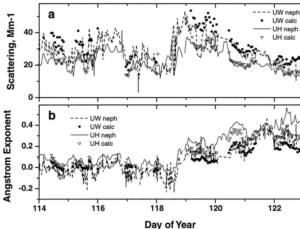
FIG. 8. Time series for (a) measured scattering and (b) the Ångström exponent determined from the UW and UH nephelometers and from corresponding size distributions corrected to nephelometer RH.
