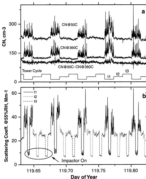
FIG. 2. A time series indicating multiple cycles through the three tower sample valves (t1, t2, t3) over a 5-h period for (top) measured CN at  $50^{\circ}$  and  $360^{\circ}\text{C}$  and their difference and (bottom) for concurrent light scattering.
