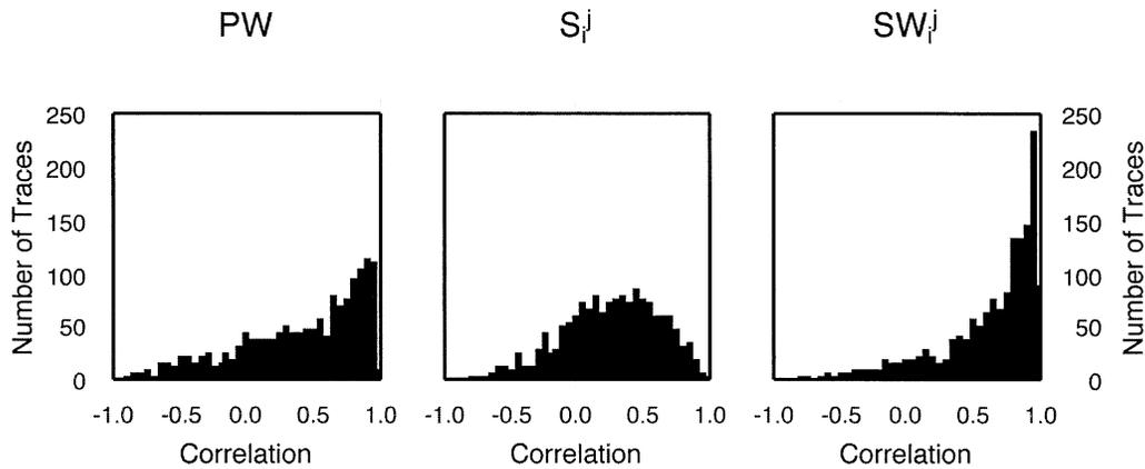
FIG. 4. Histograms of linear correlation coefficients for individual satellite traces. (left) The linear correlation of the GPS PW with respect to WVR SW, (middle) the linear correlation of  $S_i^j$  from GPS to the WVR  $S_i^j$ , and (right) the linear correlation of the GPS SW to the WVR SW.
