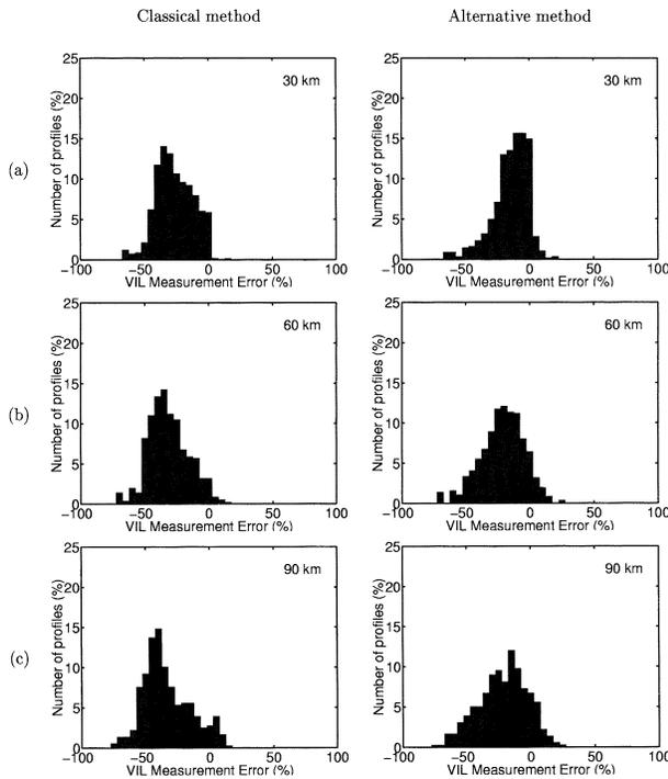
FIG. 6. VIL measurement error for convective profiles with the radar at (a) 30, (b) 60, and (c) 90 km. (left) VIL measurement error obtained using the classical method, and (right) error obtained using the alternative method. The error on the  $0^{\circ}\text{C}$ -isotherm altitude, and the density factor are distributed according to an unbiased Gaussian law, with a std dev of 200 m and 0.2, respectively.
