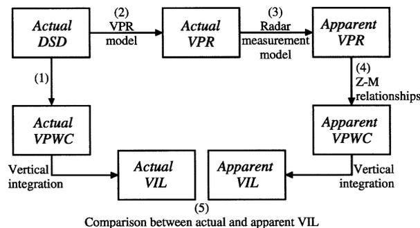
FIG. 1. Diagram of the approach adopted to estimate radar-based VIL measurement errors.
