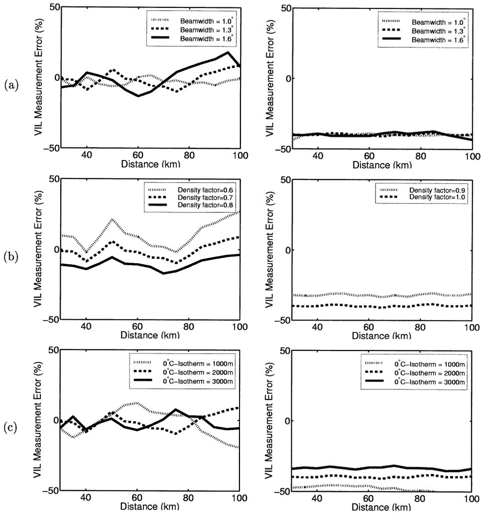
Fig. 3. Assessment of the sources of error in VIL radar measurement for reference profiles. VIL error measurement vs distance for (left) the reference stratiform profile and (right) for the reference convective profile. (a) Influence of beamwidth, (b) influence of density factor, and (c) influence of 0°C isotherm altitude.
