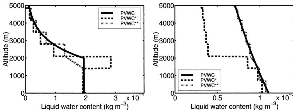
Fig. 4. Vertical profile of water content at a distance of 30 km for the (left) reference stratiform and (right) convective profile. PVWC corresponds to the actual profile, PVWC\* represents the profile obtained by the classical method, whereas PVWC\*\* corresponds to the profile obtained by the alternative method (presented in section 5).
