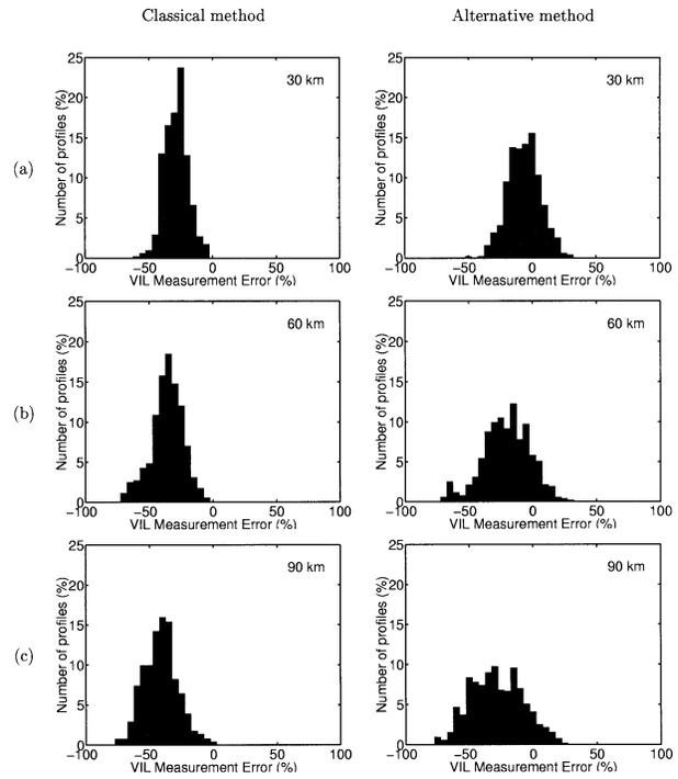
FIG. 7. VIL measurement for stratiform profiles with the radar at (a) 30, (b) 60, and (c) 90 km. (left) VIL measurement error obtained using the classical method, and (right) error obtained using the alternative method. The error on the  $0^{\circ}\text{C}$ -isotherm altitude and the density factor are distributed according to an unbiased Gaussian law, with a std dev of 200 m and 0.2, respectively.
