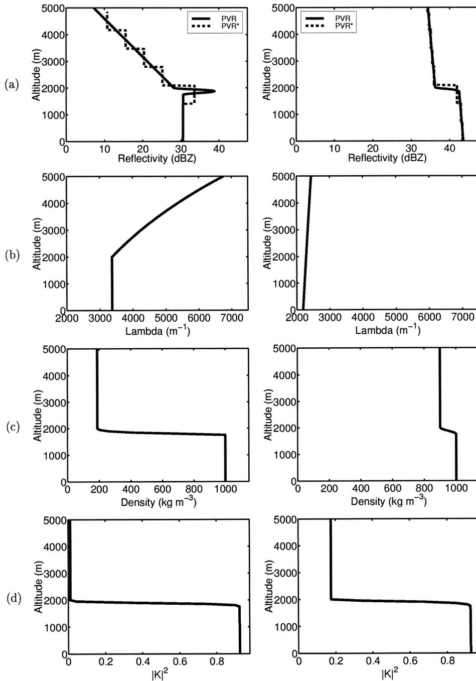
FIG. 2. Vertical profiles for the (left) reference stratiform profile,  $e = 0.7$ , and the (right) reference convective profile,  $e = 1.0$ , of (a) reflectivity, (b) second DSD parameter  $\Lambda$ , (c) mass density, and (d) dielectric factor.
