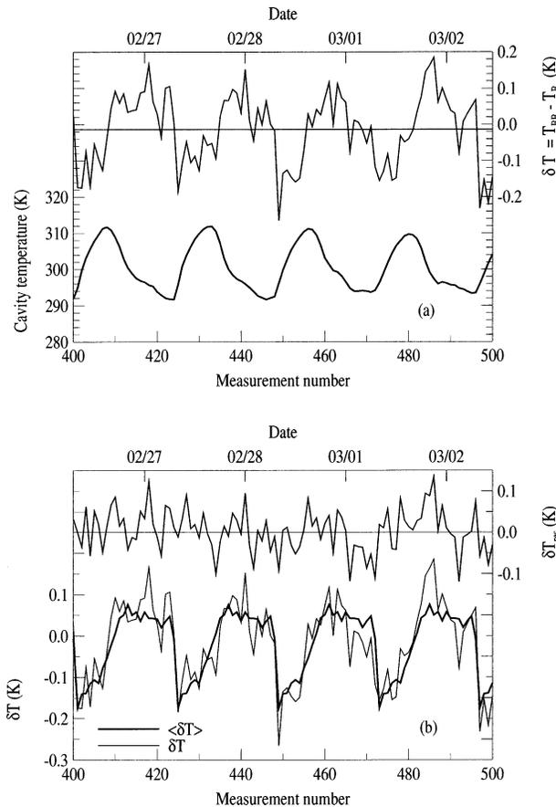
FIG. 3. [top: (a)] Comparison of the periodic behavior of the cavity temperature  $T_C$  with  $\delta T$  for a series of 100 measurements (see text). [bottom: (b)] Corresponding residual signal  $\delta T_{\text{res}}$ , which is the difference between  $\delta T$  and the solar time average value  $\langle \delta T \rangle$  of  $\delta T$ .
