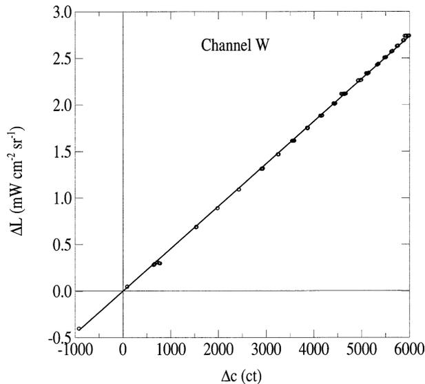
FIG. 1. Radiance calibration of channel W performed in Oct 1997 from (top right) 180 to (bottom left) 320 K,  $\Delta c$  is expressed in counts (ct). The zero value of  $\Delta c$  corresponds to the cavity temperature ( $\approx 295$  K).
