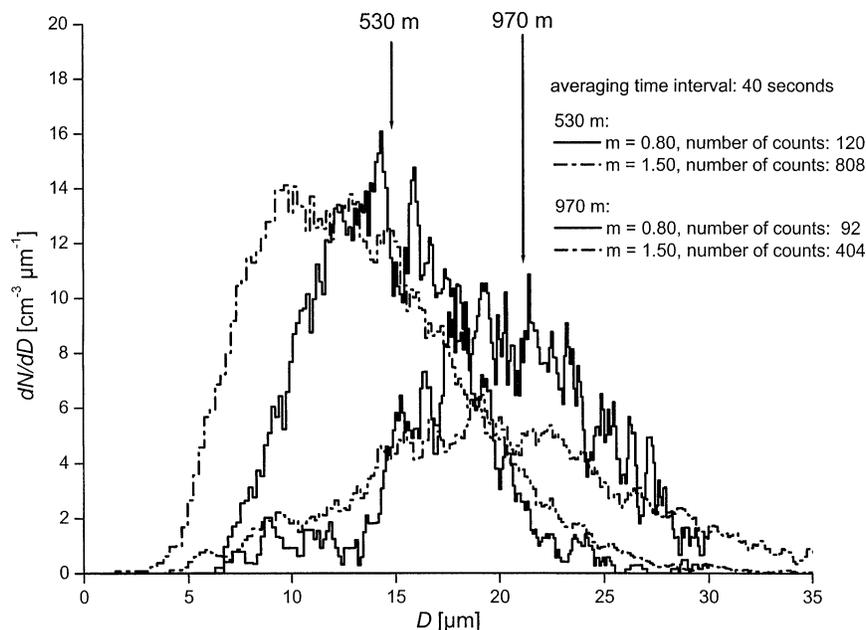
FIG. 11. BBC-2 drop size distribution at 530 and 970 m from Fig. 9 ( $m = 1.50$ : dashed-dotted line;  $m = 0.80$ : solid line). The accumulation time for all distributions is 40 seconds. The number of accumulated counts is indicated for each size distribution.
