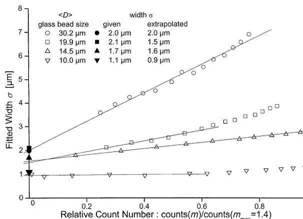
FIG. 5. Fitted width  $\sigma$  vs relative count number proportional to sampling volume (open symbols) for four different glass bead sizes with standard deviation specified by the manufacturer (plotted at zero relative count number as closed symbols). Lines are linear extrapolations to zero relative count number. Their offset is the estimated natural width of the size distribution.
