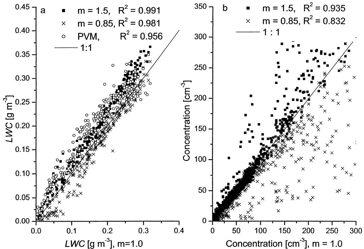
FIG. 10. BBC-2 scatterplots. (a) LWC from the PVM, M-Fast-FSSP  $m = 1.5$  and  $m = 0.8$  vs M-Fast-FSSP  $m = 1.0$ . (b) Concentration from M-Fast-FSSP  $m = 1.5$  and  $m = 0.8$  vs M-Fast-FSSP  $m = 1.0$ .
