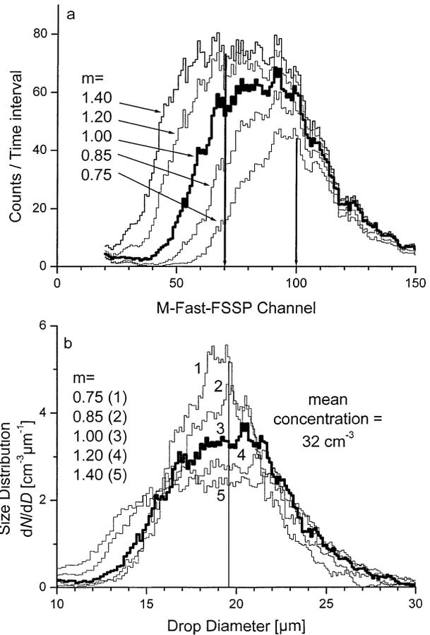
FIG. 4. (a) Channel distribution for 20- $\mu\text{m}$  glass beads; the curves with a small number of total counts correspond to low  $m$ . The higher  $m$ , the more droplets are considered to be valid and the further the maximum of the distribution moves toward lower channels. (b) Size distribution obtained by applying a calibration to (a) for each  $m$  separately.
