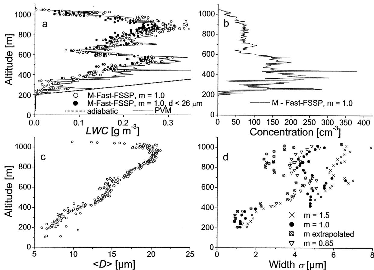
FIG. 9. BBC-2 measured altitude profiles. (a) LWC from PVM (solid line) and M-Fast-FSSP (closed circles:  $m = 1.0$ ,  $d < 26 \mu\text{m}$  only; open circles,  $m = 1.0$ , all channels); adiabatic profile (dashed line) (b) Drop concentration from M-Fast-FSSP,  $m = 1.0$ ; (c) mean diameter from M-Fast-FSSP,  $m = 1.0$ ; (d) width  $\sigma$  of drop size distribution (triangles:  $m = 0.85$ , crossed squares: extrapolated width, closed circles:  $m = 1.0$ , crosses:  $m = 1.5$ ).
