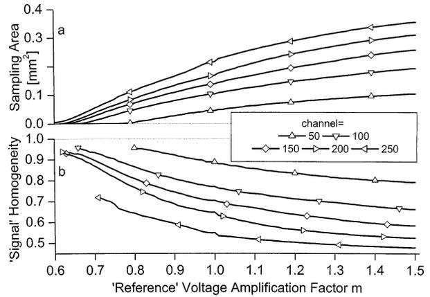
FIG. 3. Sampling area and Signal homogeneity: (a) sampling area as function of the Reference amplification factor  $m$  for five different channels and (b) Signal homogeneity defined as average of the Signal voltage within the sampling area normalized to its maximum value as function of  $m$ .
