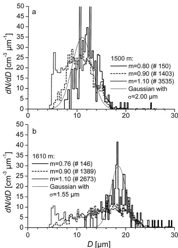
FIG. 7. INSPECTRO drop size distribution at two altitudes from Fig. 6.  $m = 0.76/0.80$ : solid line,  $m = 0.90$ : dashed line,  $m = 1.10$ : dotted line. (a) At 1500 m, (b) at 1610 m. The accumulation time for all distributions is 10 s. The number of accumulated counts is indicated for each size distribution (#). The thin line is a Gaussian with the extrapolated width.
