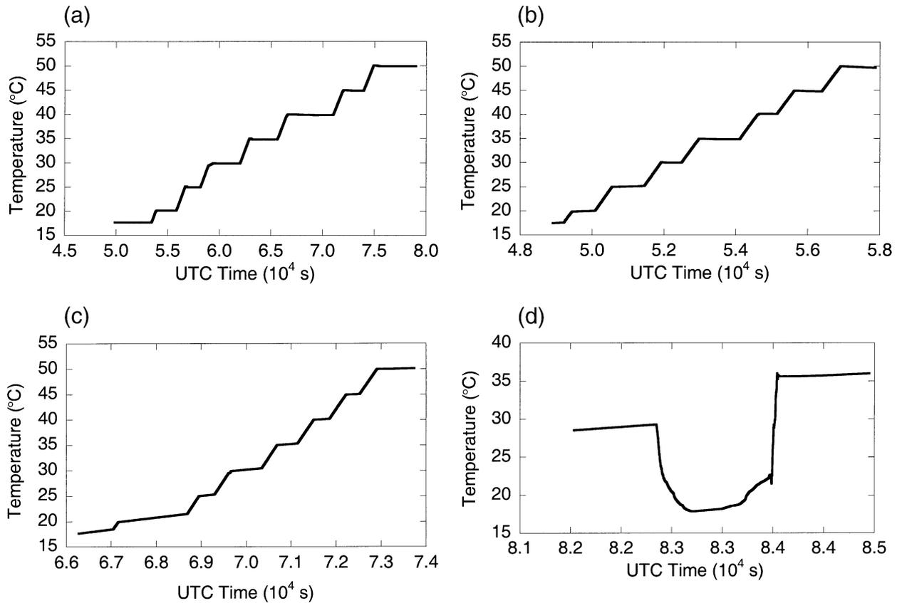
FIG. 4. Contact temperature ( $T_c$ ) vs time data for each of the blackbodies tested. The temperature sweeps were from lowest to highest temperature. On this scale, brightness temperature data taken simultaneously in both channels of the TXR lay on top of the contact temperature and are not plotted. Only data near the end of each plateau were used for the analysis as described in section 7: (a) RSMAS blackbody, (b) JPL blackbody, (c) CASOTS RAL blackbody, and (d) CASOTS SOC blackbody.
