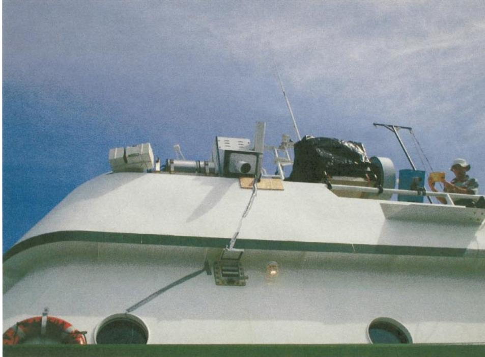
FIG. 3. The infrared radiometers mounted on the upper deck. From the left these are SISTeR, ISAR-5, CIRIMS, M-AERI, DAR011, and the hand-held TASCO. The JPL radiometer was mounted on the foredeck, viewed the sea between the two hulls of the *Walton Smith*, and is not visible in this photograph.
