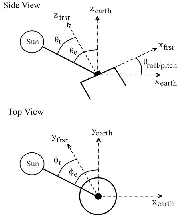
FIG. 1. The geometry of a shadow-band radiometer operated on a moving platform.
