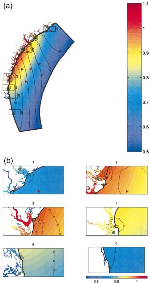
FIG. 5. (a) The M2 tidal solution on Peach2 mesh, prior to inversion. The color shading interval for the amplitude (m) represents 1 cm and the contour interval for the phase isolines is  $3^\circ$ . (b) Prior M2 solution on the Peach2 mesh: detail at the operational stations. Figures 5, 6, 8 and 9 follow the same convention.
