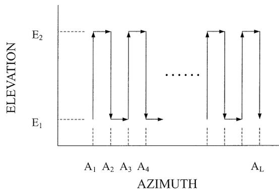
FIG. 1. Track of vertical antenna scan in an azimuth sector.
