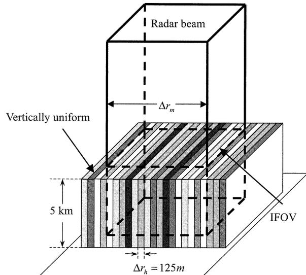
FIG. 2. Schematic diagram of rain cell sensing by a spaceborne radar.
