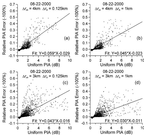
FIG. 7. Scatterplot of the relative PIA NUBF error vs the uniform PIA obtained from the same rain data as those in Fig. 3. The straight line is a linear fit with its equation given. The IFOV sizes are (a) 4, (b) 4, (c) 3, and (d) 3 km. The resolutions of data used are (a) 0.125 (high), (b) 1 (low), (c) 0.125, and (d) 1 km.
