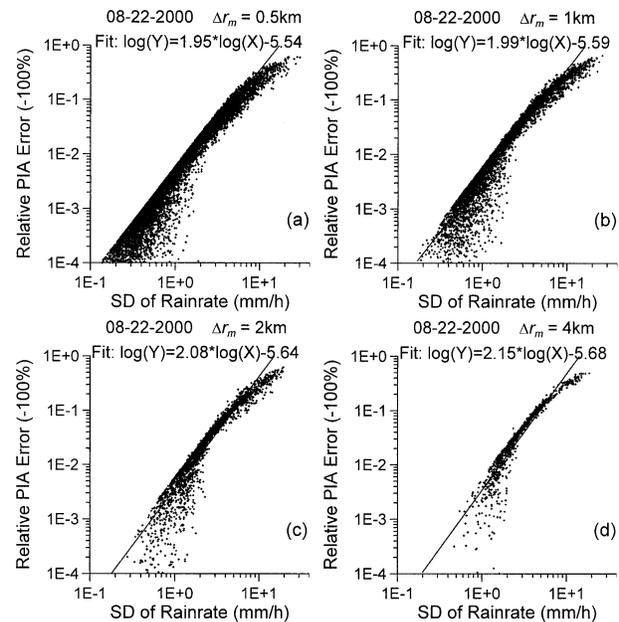
FIG. 6. As in Fig. 4 except for the relative PIA NUBF error vs the SD of rain rate.
