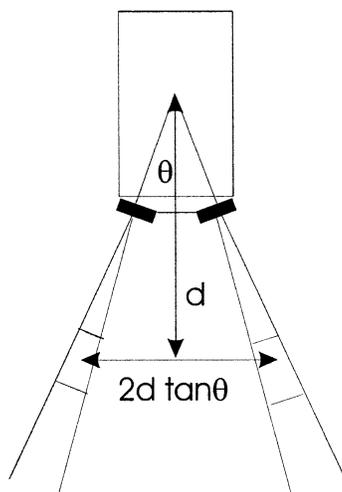
FIG. 1. Schematic of the ADCP beams showing the variables defined in the text.
