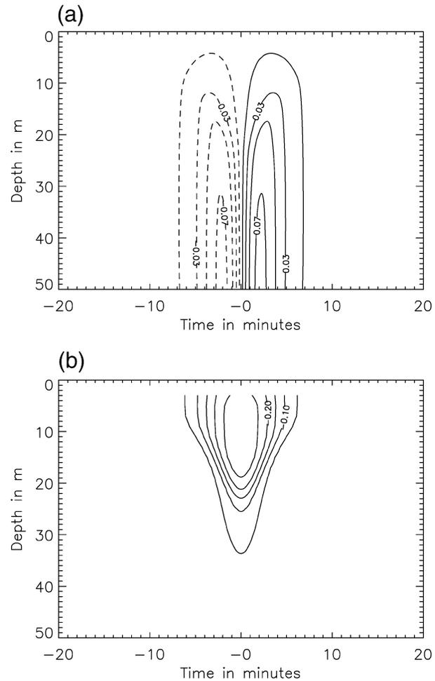
FIG. 2. Contour of simulated (a) vertical ( $w$ ) and (b) anomaly horizontal ( $u$ ) velocity fields. For (a) the dashed and solid lines represent downward and upward flows, and the contour interval is 0.02 m s<sup>-1</sup>. In (b) the contour interval is 0.05 m s<sup>-1</sup>.
