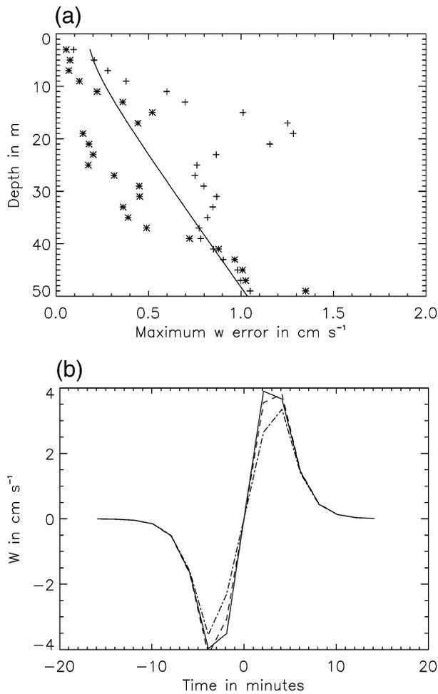
FIG. 3. (a) Maximum absolute error of the uncorrected (crosses) and corrected (stars) estimates of the vertical velocity as a function of depth. (b) The unconvolved (solid), convolved (dot-dashed), and corrected (dashed line) waves as a function of time at 17-m depth.
