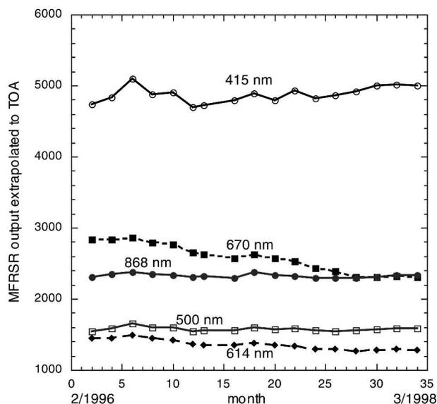
FIG. 6. Time series of calibration values in counts for five channels of the Multifilter Rotating Shadowband Radiometer deployed at the Bondville SURFRAD station from Jan 1996 through Mar 1998.
