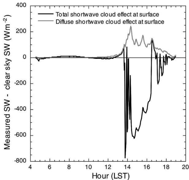
FIG. 5. Time series of the effect of clouds on surface shortwave radiation at the Table Mountain SURFRAD station for 21 Jun 2004. The black solid curve is the difference between measured and clear-sky total solar in Fig. 4, and the gray curve is the difference between measured and clear-sky diffuse in Fig. 4.
