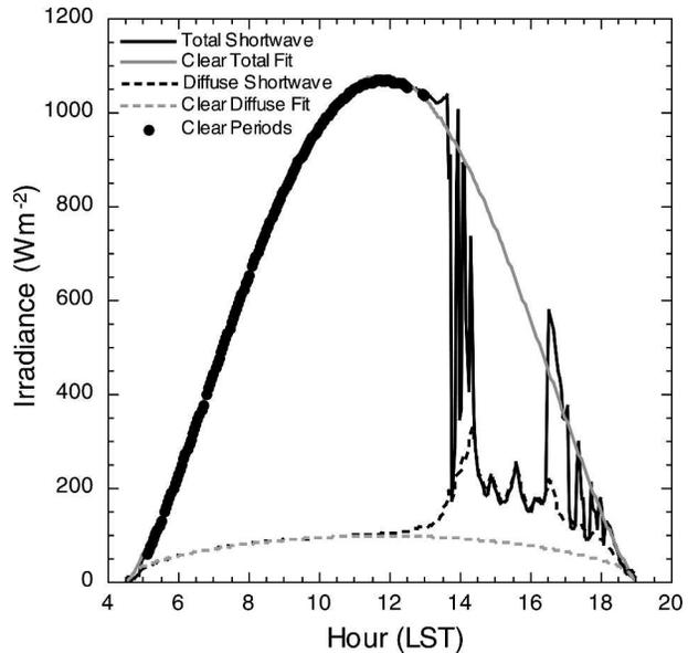
FIG. 4. Measured total solar (solid black) and diffuse (dashed black) irradiance, and clear-sky envelopes (gray) for those parameters for the Table Mountain SURFRAD station on 21 Jun 2004. Black dots indicate times determined to be cloud free by the Long and Ackerman (2000) clear-sky identification algorithm.
