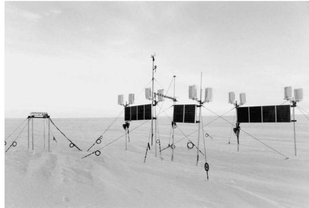
FIG. 2. Photograph of the Doppler sodar wind profiling system after installation in 2001/02. The photo is looking toward the southwest. In the foreground is the sodar antenna; to the right are the three rows of solar panels, the wind generators, and the radio antenna. To the left is the mast of the AWS.
