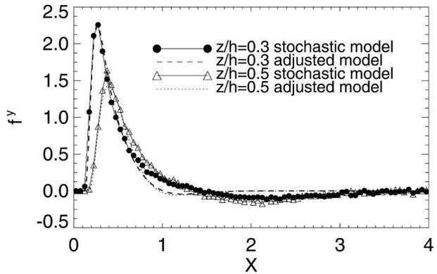
FIG. 3. Comparison of the footprints (CWIF) calculated from the adjusted model and from the stochastic model for measurement heights of 0.3 and 0.5h in the case of  $L/h = -0.03$  and roughness length  $= 1 \times 10^{-3}h$ .
