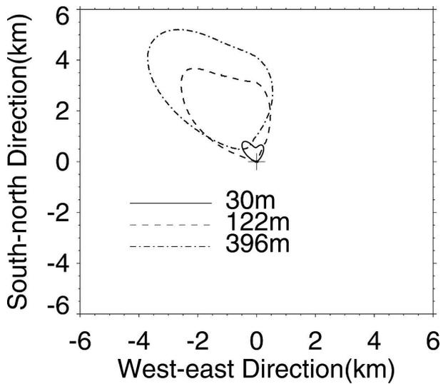
FIG. 5. The 80% surface source (sampling) areas for flux measurements at three heights of 30, 122, and 396 m, respectively. The cross represents the location of the tower. The three lines represent the 80% surface source area boundaries, estimated using the averaged footprint with meteorological conditions measured at the WLEF tower from 0900 to 1700 local time 4 Jun 1998. A dynamically homogeneous surface is assumed in this example.
