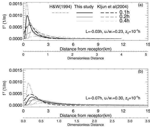
FIG. 4. Comparison of the estimated CWIFs from the adjusted model of this study [Eq. (17)] (solid lines) and from the empirical model (broken lines) by Kijun et al. (2004) at three heights above the surface layer with (a)  $L = -0.03h$  and (b)  $L = -0.07h$  for  $z_0 = 10^{-4}h$ . The dot-dash lines are the results at the top of the surface layer (0.1h) from the analytical surface layer model by Horst and Weil (1994).
