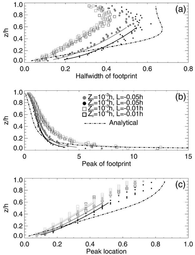
FIG. 2. Normalized (a) half-width, (b) peak, and (c) peak's location of CWIF derived from the idealized model (dot-dash lines) as a function of dimensionless measurement height ( $z/h$ ). Results from the stochastic model are shown by circles and squares, suggesting the dependence of the quantities on  $L/h$  and  $z_0/h$ . The solid lines are the fitted lines for the three quantities. Limited horizontal resolution of the stochastic model results in "steps" in (c).
