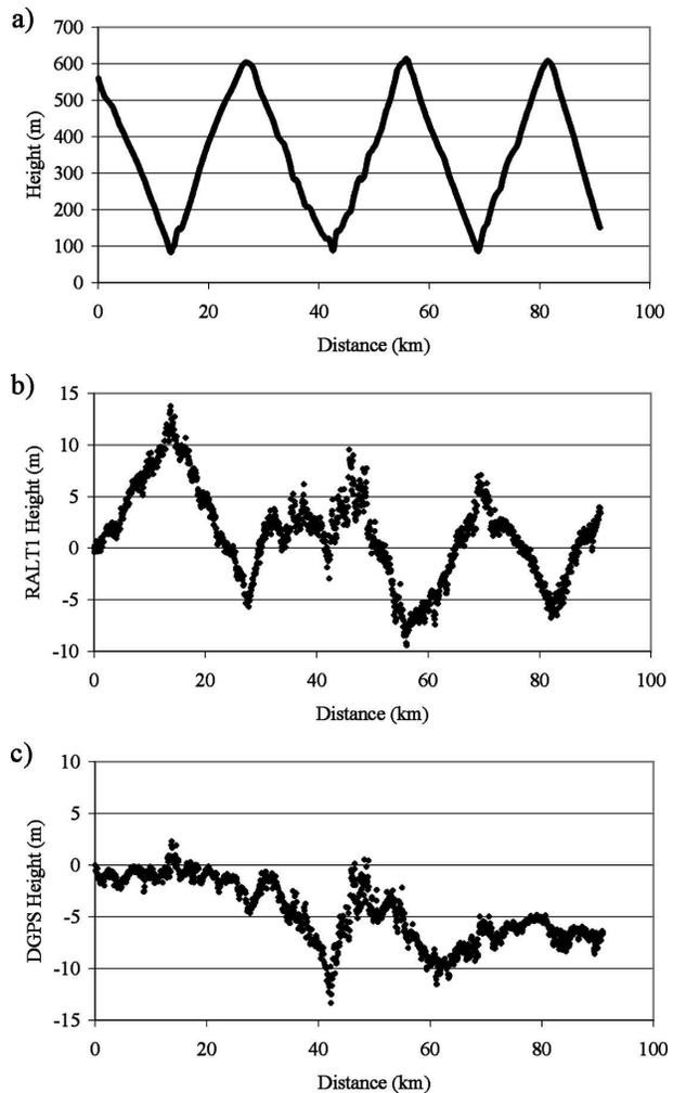
FIG. 2. Flight data from 04 Oct 2004 showing (a) heights (m) and height differences (m) between hydrostatically calculated values, and (b) RALT1 and (c) DGPS heights.
