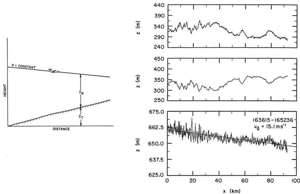
FIG. 1. (left) Schematic of horizontal pressure gradient force determination and (right) examples from Parish et al. (1988). At left,  $Z_T$  refers to the terrain height above sea level, and  $Z_R$  is the height above the terrain as measured by radar altimeter. At right, (top) radar altimeter signal, (middle) inferred underlying terrain height, and (bottom) isobaric surface height above sea level.
