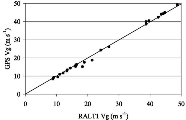
FIG. 5. Comparison of geostrophic wind ( $\text{m s}^{-1}$ ) determination from RALT1 and differential GPS height measurements for 28 legs taken from ROLLS04 (January 2004), GPS04 (June 2004), and GOA04 (October 2004). Straight line represents 1:1 fit.
