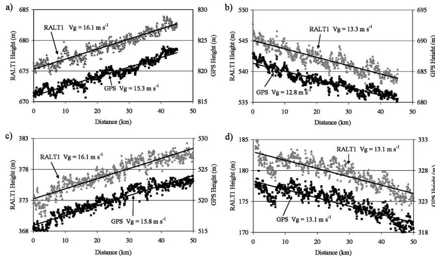
FIG. 3. The 1-Hz heights of mean isobaric surfaces of (a) 911, (b), 929, (c) 949, and (d) 975 hPa for four consecutive legs from UWKA flights on 22 Jan 2004 from RALTI and differential GPS. Here  $V_g$  indicates equivalent geostrophic wind speeds, and straight lines represent least squares linear fit.
