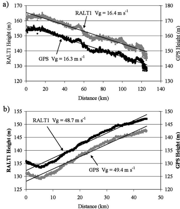
FIG. 4. Heights of isobaric surfaces derived from RALT1 and differential GPS measurements for (a) 5 Oct 2004 and (b) 22 Jun 2004. Straight lines represent least squares linear fit.
