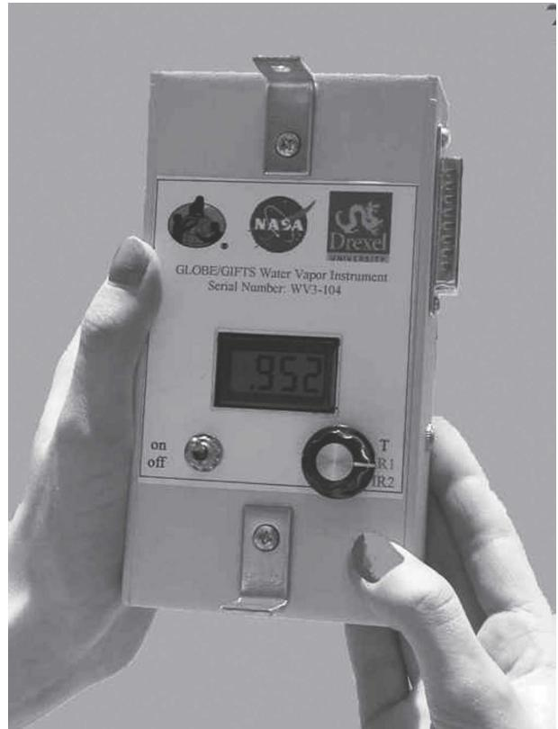
FIG. 3. GLOBE water vapor instrument.
