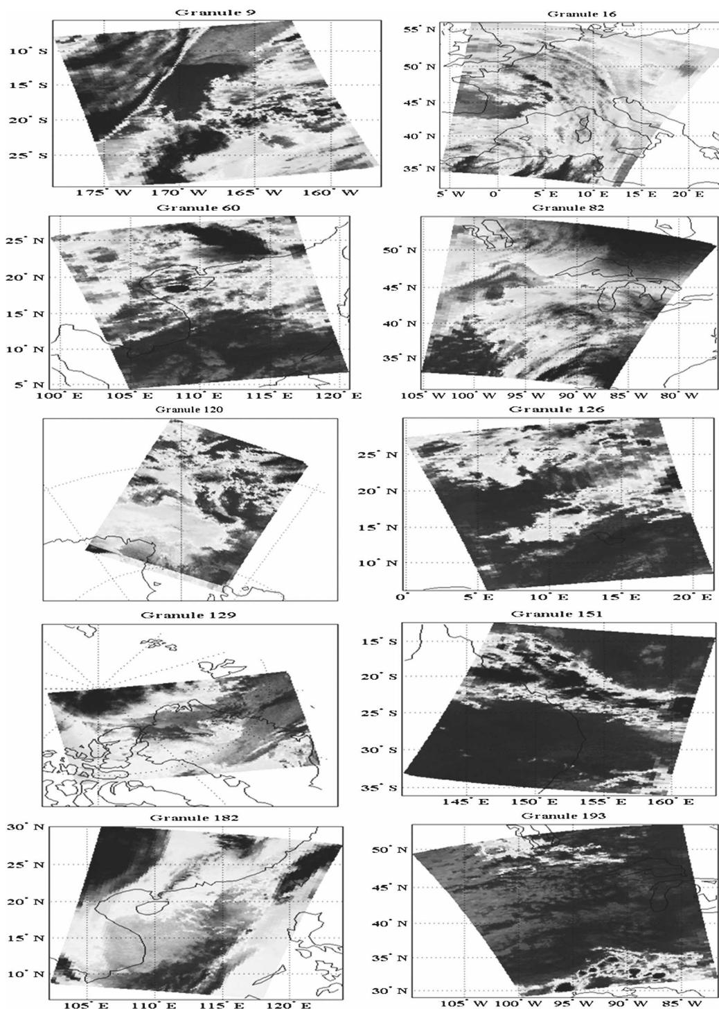
FIG. 1. AIRS digital counts at wavenumber  $800.01 \text{ cm}^{-1}$  for the 10 selected granules on 2 Mar 2004.
