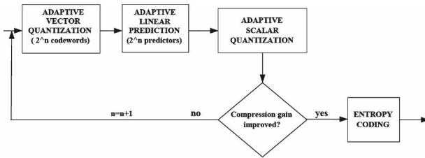
FIG. 2. Block diagram of the AVQLP method.
