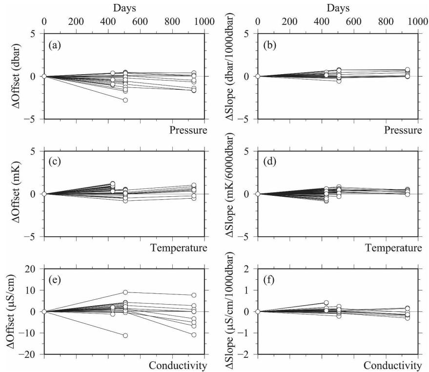
FIG. 5. Accumulated drift after the first in situ calibration of the SBE-37s. Offset is defined here as the difference between the SBE-37 and shipboard CTD data at 4500 dbar estimated from the in situ calibration coefficients. The slope is the same as that in Fig. 3.
