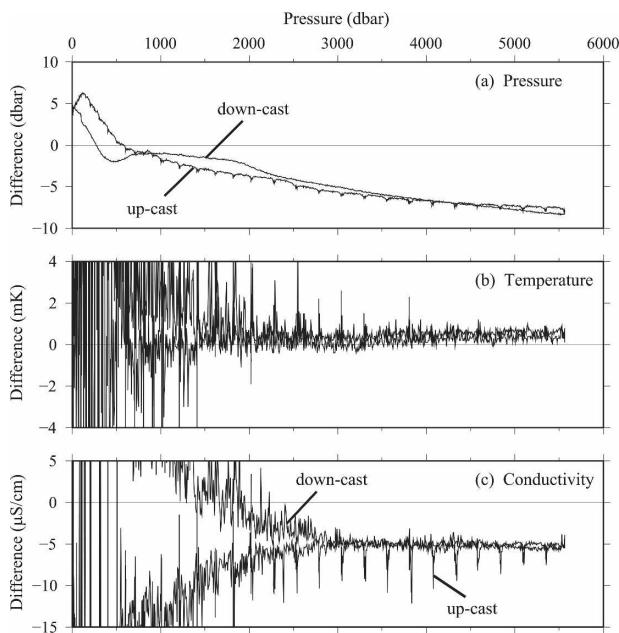
FIG. 2. An example of differences in pressure, temperature, and conductivity between an SBE-37 (No. 24 in Fig. 3) and the shipboard CTD. The SBE-37 data, sampled at 6-s intervals, were compared with the shipboard CTD data averaged over 1 s for down- and upcasts.
