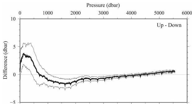
FIG. A1. Mean pressure difference (thick line) between the up- and downcasts of the in situ calibrations for 42 SBE-37s before mooring deployment. Thin lines represent one standard deviation from the mean.
