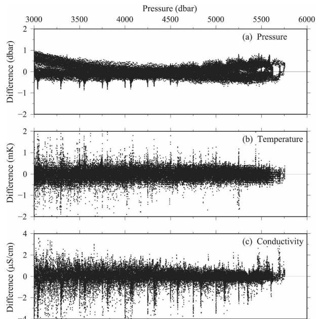
FIG. 4. Differences between SBE-37 and shipboard CTD data plotted against pressure. Results of the in situ calibration before mooring deployment of the 50 SBE-37s are shown for pressure, temperature, and conductivity.
