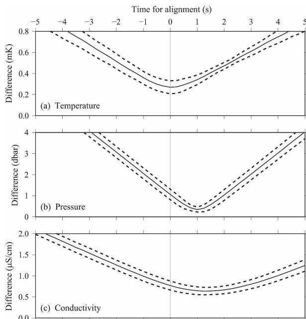
FIG. 1. Differences between the SBE-37 and shipboard CTD data for depths deeper than 3000 dbar, from down- and upcasts. Mean (solid line) and standard deviation (dashed lines) of root-mean-square differences from a fitted line are calculated from 25 comparisons on the R/V *Mirai* cruise MR03-K02. Differences for temperature, pressure, and conductivity are shown as a function of time for alignment of the SBE-37 data, relative to minimizing time of the temperature difference.
