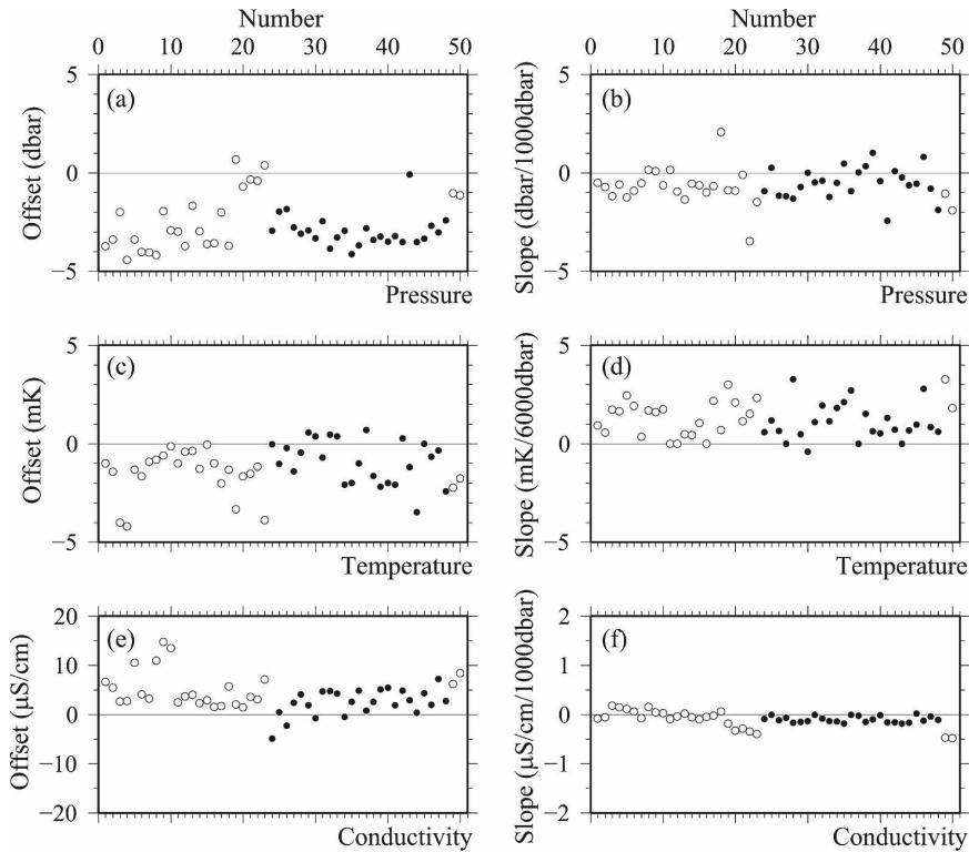
FIG. 3. Calibration coefficients obtained from comparisons between SBE-37s and shipboard CTDs before mooring observation plotted against the sequential number of the 50 SBE-37s. Filled circles show results from May 2003 and open circles show results from October 2004.
