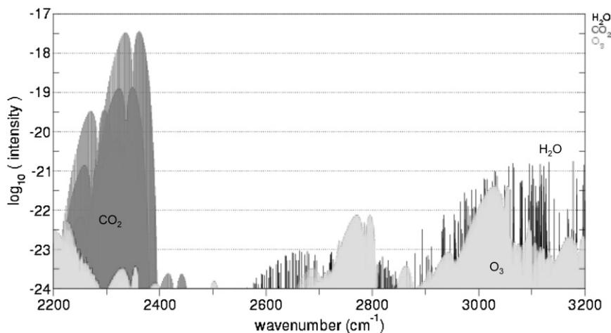
FIG. 3. Absorption line strengths of CO<sub>2</sub> (dark gray), H<sub>2</sub>O (black), and ozone (light gray) between 2200 and 3200 cm<sup>-1</sup>. Data are from SpectralCalc.com.
