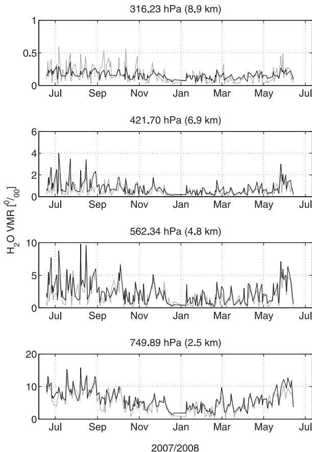
FIG. 4. Time series of  $\text{H}_2\text{O}$  mixing ratio as measured by RS92 (gray lines) and the ground-based microwave radiometer (black lines) at four different pressure levels. RS92 profiles have been corrected for the radiation dry bias (see section 4).
