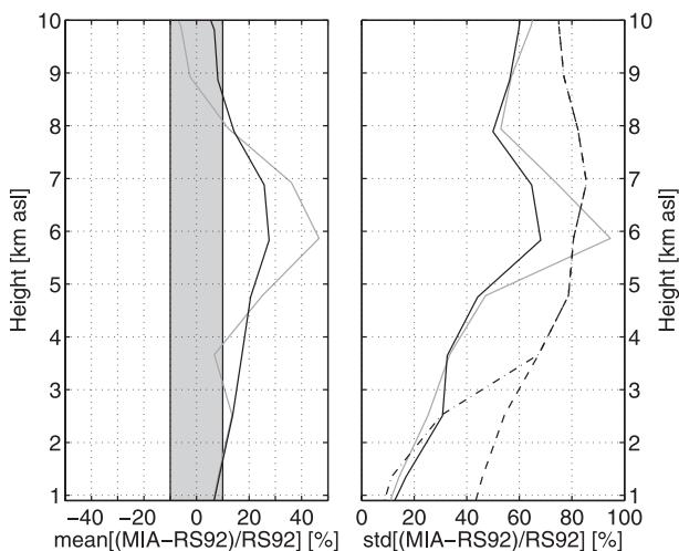
FIG. 5. (left) Mean and (right) std dev of the relative differences between the radiometer (MIAWARA) and RS92 profiles considering only measurements after 1 Oct 2007 (solid black line; 145 profiles) and considering all measurements (solid gray line; 203 profiles). (right) The natural variability of water vapor (dashed line) and the random error of the a priori (dashed-dotted line) are also displayed.
