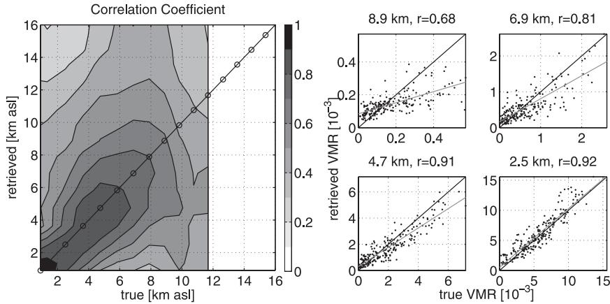
FIG. 2. Analysis of the simulated retrievals. (left) Matrix of correlation coefficients between the true and the retrieved profiles. Because the true profiles are based on RS92 measurements, they are only taken into account up to 11.5 km. (right) Scatterplots of the true and the retrieved data, where  $r$  is the correlation coefficient.
