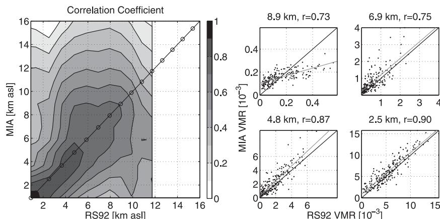
FIG. 3. Analysis of the real retrievals. (left) Matrix of correlation coefficients between RS92 and the microwave retrievals (MIAWARA). RS92 measurements are only taken into account up to 11.5 km. (right) Scatterplots of RS92 and radiometer data, where  $r$  is the correlation coefficient. RS92 profiles have been corrected for the radiation dry bias (see section 4).
