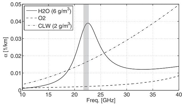
FIG. 1. Absorption coefficient between 10 and 40 GHz at 850 hPa for water vapor, cloud liquid water, and oxygen. The shaded area marks the bandwidth of the radiometer.
