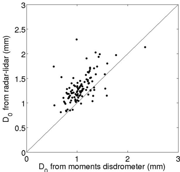
FIG. 6. Reference drop size  $D_0$  from in situ disdrometer measurement vs lidar-radar estimation.
