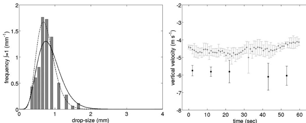
FIG. 5. (left) Example of an RSD measured by a disdrometer and estimated gamma distribution based on the first three moments of the disdrometer measurement (dashed line) and on the method using the radar–lidar combination (solid line). (right) Corresponding raindrop fall velocities show the difference between lidar (gray dots) and radar (black squares) measurement (error bars due to variations along range gates).
