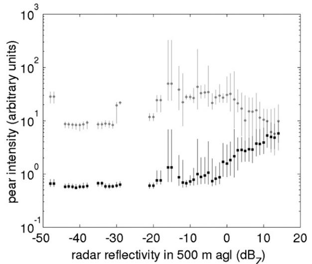
FIG. 3. Comparison of the peak intensity of the two peaks in the lidar Doppler spectra and radar reflectivity. Gray dots represent the aerosol peak and black squares are the rain peak. Vertical lines show the 25th–75th percentile and the symbols show the 50th percentile.
