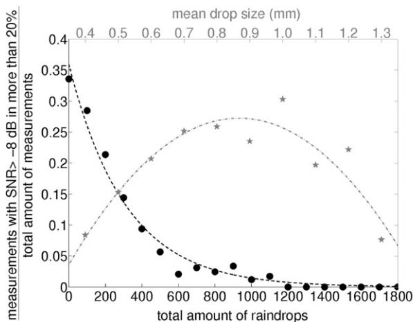
FIG. 1. Fraction of reliable velocity measurements as a function of the total amount of raindrops (black dots) and the mean raindrop size (gray stars).
