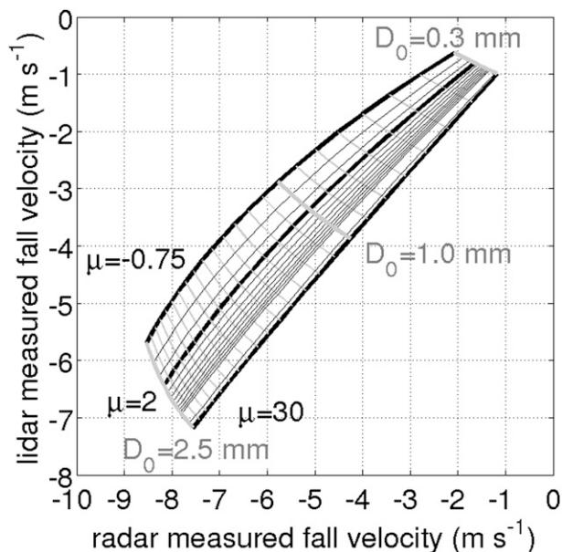
FIG. 4. Effect of a variation of the rain velocity measured by radar and lidar on the parameters  $\mu$  (black) and  $D_0 = (\mu + 4)/\lambda$  (gray).
