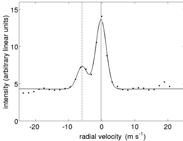
FIG. 2. Lidar Doppler spectra during light rain (dots) and with a Gaussian model (thick solid line). Two peaks could be observed: an aerosol peak (right) and a rain peak (left). The automatic lidar algorithm always detects the higher peak, while the Gaussian model detects both peaks.
