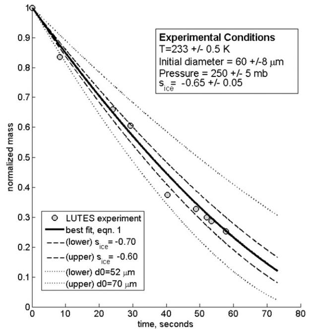
FIG. 4. Sublimation measurements of decreasing mass, normalized to the initial particle mass  $m_0$  (circles) and particle model [(2), solid line] for  $\text{LN}_2$  frozen ice particles at  $-40^{\circ}\text{C}$ . The bracketing curves express (2) given deviations in  $s_{\text{ice}}$  (dashed) and initial particle diameter (dotted).
