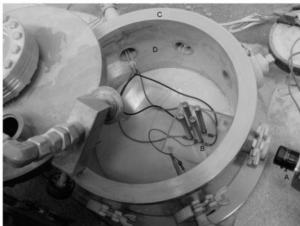
FIG. 2. The levitation cell and vacuum chamber inside the So-Low freezer.
