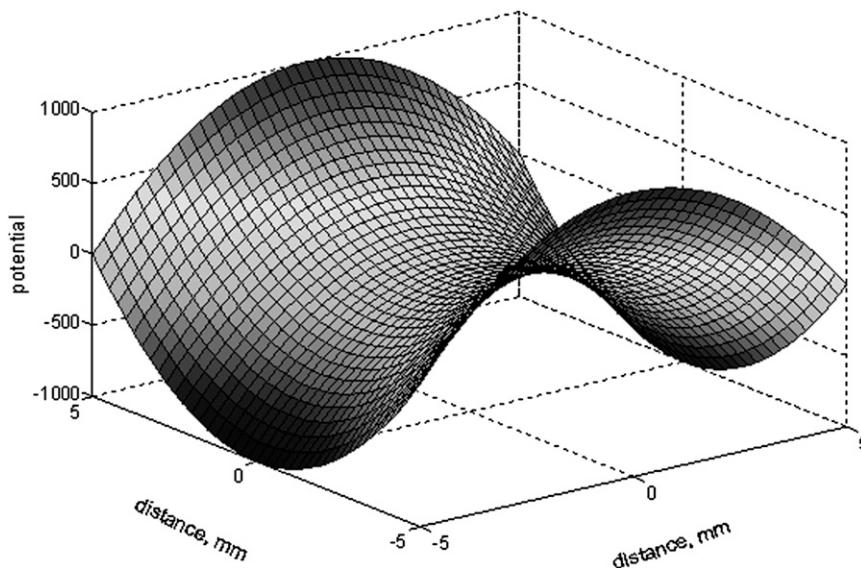
FIG. 3. Saddle AC electric potential along the horizontal plane through a levitated ice particle. For a complete theoretical treatment of the quadrupole EDB plus one levitation configuration, please see Hu and Makin (1991).
