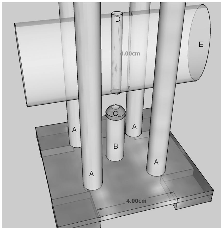
FIG. 1. Diagram of quadrupole plus one EDB including zone of levitation (thin vertical cylinder) and optical pathway for lighting and video (cylinder of elliptical cross section). The cylindrical vertical electrodes are  $\frac{3}{8}$ -in. polished stainless steel. The detachable particle collection cup is shown atop the short central electrode.
