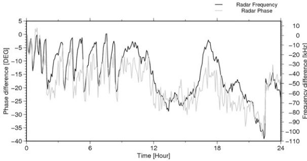
FIG. 4. Time series, for 16 Mar 2010, of the phase difference  $\Delta\Phi_{2,1}(t, t_{\text{ref}})$  of two signals coming from the same isolated target sampled at two successive range gates (gray line). The reference time  $t_{\text{ref}}$  is fixed to the first available time of the day. Time series of the transmitted signal magnetron frequency difference  $[f(t) - f(t_{\text{ref}})]$  (black line, right scale in kHz).
