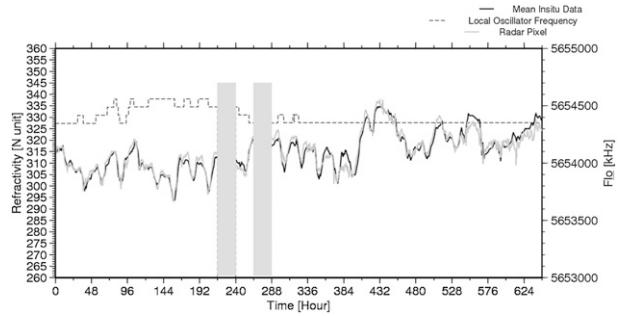
FIG. 5. Time series of refractivity  $N$  measured by the radar during a 27-day period (2–30 Mar 2010) for the radar pixel. Averaged refractivity measurements from the three AWS (solid black line). Local oscillator frequency (right scale, dashed line). The two gray columns indicate no data and the time  $t_{\text{ref}}$  is reset after each period of absence of data.
