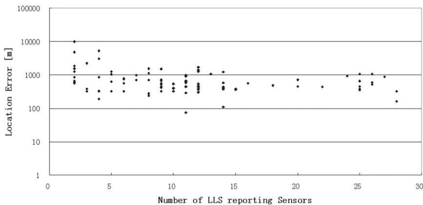
FIG. 5. Absolute location error vs number of LLS reporting sensors for 96 strokes observed in triggered lightning and natural lightning during 2007–11.
