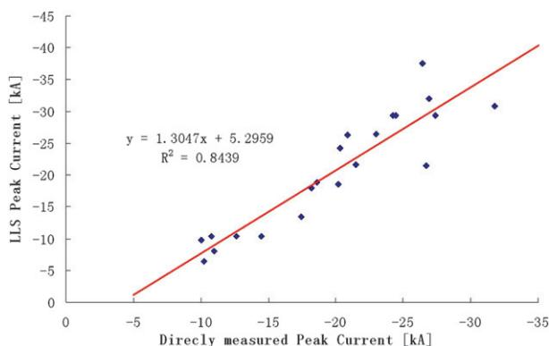
FIG. 6. LLS-reported vs directly measured peak currents in the triggered lightning experiment.
