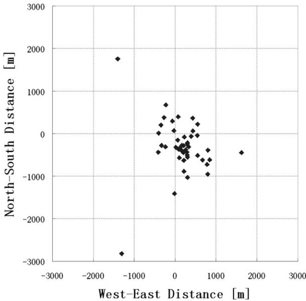
FIG. 4. Plot of 54 natural lightning stroke locations at tall structures during 2009–11. The origin corresponds to the ground strike point.
