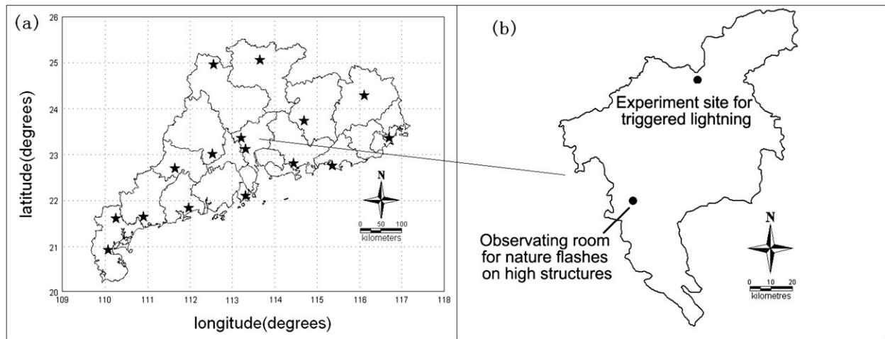
FIG. 1. Distribution of (a) sensors at the Guangdong power grid LLS and (b) observation experiment sites for lightning.
