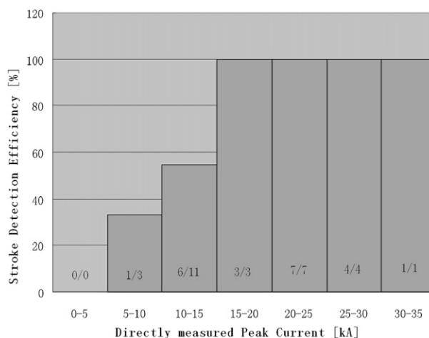
FIG. 2. Stroke detection efficiency as a function of peak current measured directly in the triggered lightning experiment. The ratio given inside the column indicates the number of strokes detected by the LLS (numerator) and the number of strokes recorded in the triggered lightning experiment (denominator).
