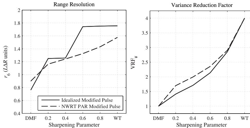
FIG. 4. (left) Range resolution ( $r_6$ ) and (right) variance reduction factor ( $VRF_\infty$ ) for cases A and B, including a DMF, a WT, and pseudowhitening transformations with varying sharpening parameter  $\alpha$ . An idealized modified pulse (solid line) and the modified pulse of the NWRT PAR (dashed line) are shown.
