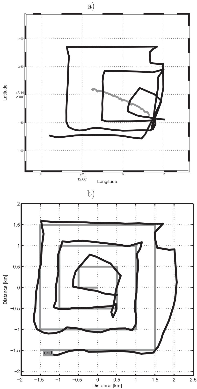
FIG. 3. As in Fig. 2, but for the expanding square spiral test during the Latex00 cruise. Discrepancies are again observed near turn points  $(-0.5, 0.5)$ ,  $(0.5, -0.5)$ ,  $(1, 1)$ , and  $(1.5, 1.5)$ .
