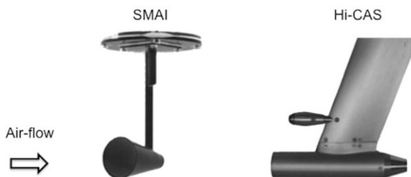
FIG. 1. Pictures of the SMAI (Craig et al. 2013b) and Hi-CAS flow-restriction inlets.
