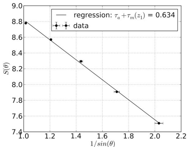
FIG. 1. Representative single measurement showing a range-corrected lidar signal  $S(\theta)$  vs air mass  $1/\sin(\theta)$ . The data were taken at 2252 UTC 26 Feb 2013 in El Segundo,  $z_1 = 15$  km, and the coefficient of determination of the regression is  $R^2 = 0.9984$ .
