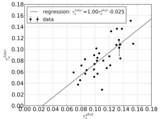
FIG. 3. Scatterplot of lidar AOT vs time-coincident sun photometer AOT at 355 nm for the campaign from 13 to 28 Feb 2013 in El Segundo;  $R^2 = 0.55$ .
