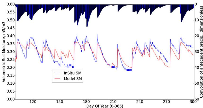
FIG. 2. Freeport 2014. Model vs dielectric probe in situ.
