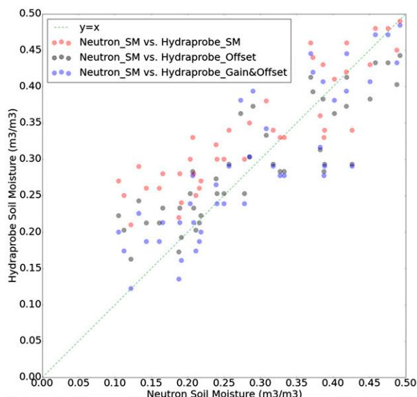
FIG. 3. Fairfield 2003–08. Dielectric probe vs neutron probe comparisons.
