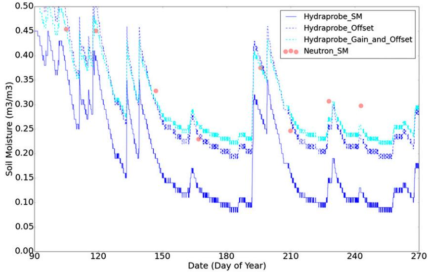
FIG. 4. Carbondale 2005. Illustration of adjusted dielectric probe data to approach neutron probe measurement values.
