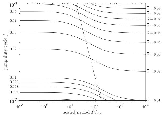
FIG. 3. Contours of mean scaled temperature  $\bar{\theta}$  as a function of the fraction of time the sensor jumps out of the water and the period  $P/\tau_{oc}$  scaled by the adjustment time scale of the sensor in water. The dashed line shows  $r_{air} = fP/\tau_{air} = 1$
