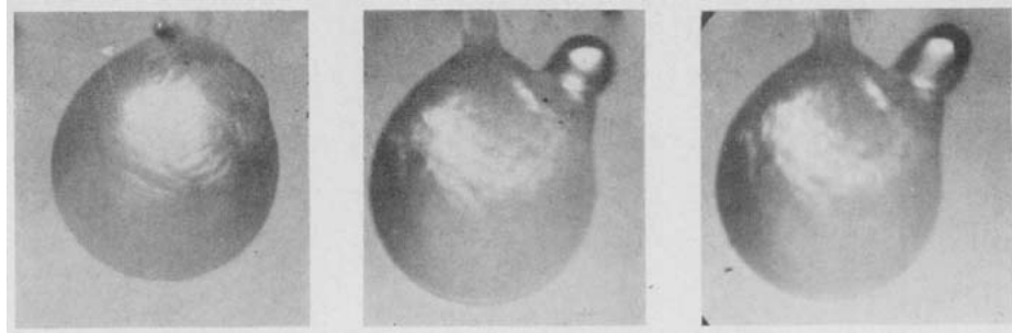
FIG. 2. Successive photographs of freezing of a water droplet in air.
