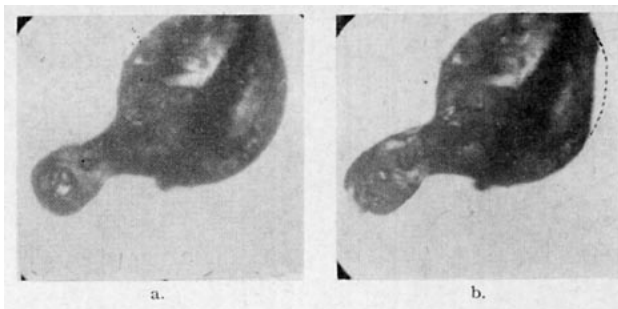
FIG. 5. Freezing of a droplet in 30% of carbon dioxide showing formation of a spike, a., and partial fragmentation, b.
