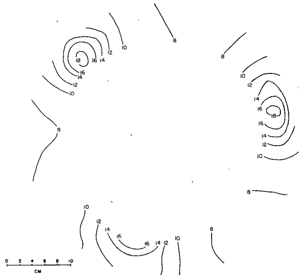
FIG. 5. Surface deficit pressure fields over a limited area for three successive subsidiary vortices. S = 2.45 , Re_r = 2.90 \times 10^4 , a = 0.6 . Units of deficit pressure are Pascals.
