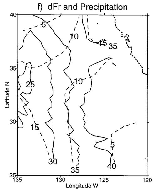
FIG. 15. (f) CTBL radiative flux divergence  $\Delta F_R$  (solid) and scaled surface precipitation rate  $-\rho_{ref}LF_p(0)$  (dash) in  $\text{W m}^{-2}$  (divide by 30 to obtain precipitation rate in  $\text{mm day}^{-1}$ ).
