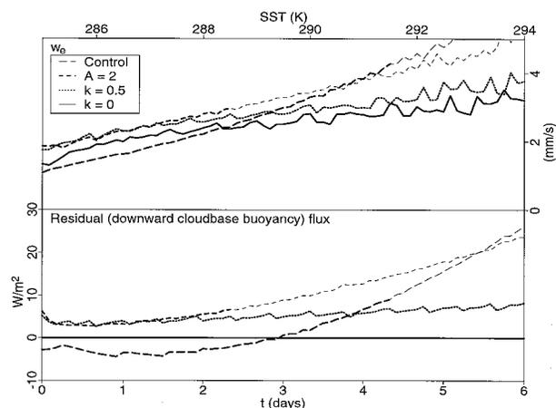
FIG. 10. Entrainment rate (top) and residual flux (bottom) for the four entrainment closures: Control (TN87 with variable  $A$ ), TN87 with fixed  $A = 2$ , Schubert flux-partitioning closure with  $k = 0.5$ , and energy balance closure ( $k = 0$  curve). Lines are thickened while MLM remains coupled ( $\text{BIR} < 0.15$ ).
