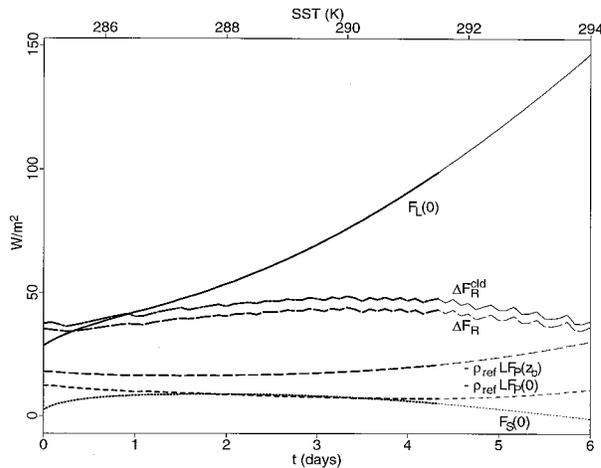
FIG. 5. Time series for the control run of surface latent heat flux  $F_L(0)$  and sensible heat flux  $F_S(0)$ , radiative flux divergence integrated across the cloud ( $\Delta F_R^{\text{cl}}$ ) and across the CTBL ( $\Delta F_R$ ), and precipitation fluxes at the cloud base ( $F_p(z_b)$ ) and surface ( $F_p(0)$ ), both scaled into units of heat flux. Lines are thickened while MLM remains coupled ( $\text{BIR} < 0.15$ ).
