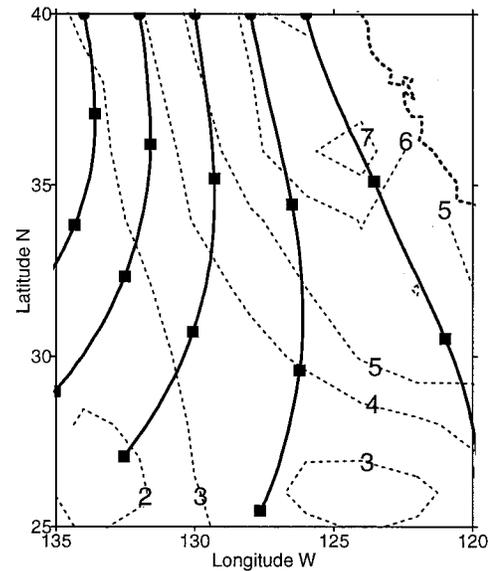
FIG. 15. (a) July climatological trajectories (solid) used in northeast Pacific MLM integrations and horizontal divergence (dash, units of  $10^{-6} \text{ s}^{-1}$ ). Heavy dashes indicate coastline. Half-octagons indicate starting location of air columns, and squares indicate air-column positions at 1, 2, and 3 days.
