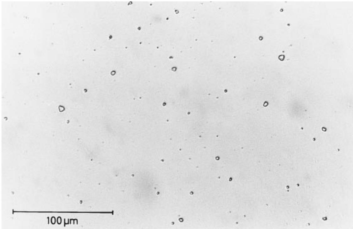
FIG. 5. An example of crystal replicas from the flight on 18 March 1994.
