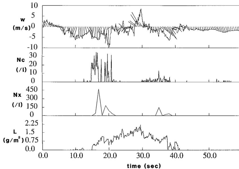
FIG. 3. Time series of data gathered on 10 August 1987. (a) The vertical wind and wind vectors constructed from the vertical wind and the horizontal wind component along the flight track; (b) the concentration of particles detected by the 2DC probe; (c) concentration of particles measured by the 260X probe; and (d) the liquid water content measured by the Forward Scattering Spectrometer Probe (FSSP).
