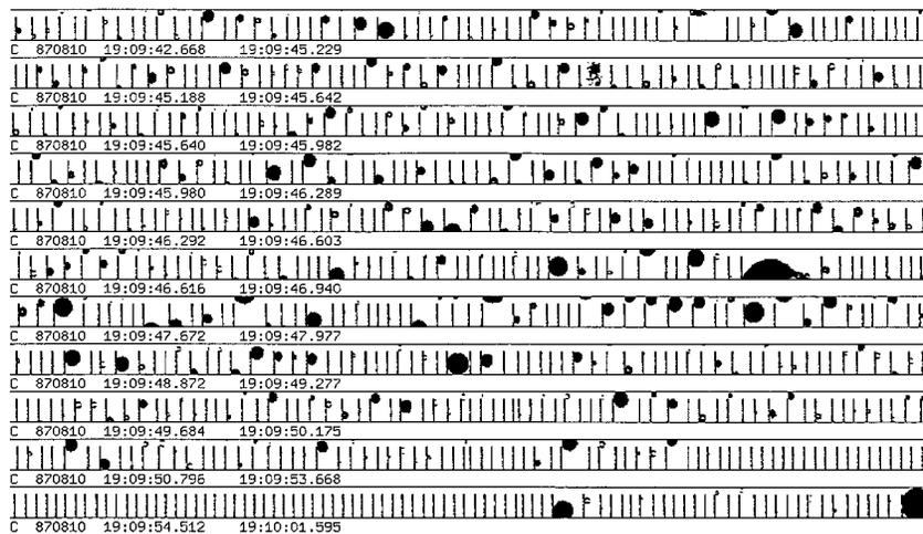
FIG. 2. 2D images made with the 2DC probe at 1909:45 on 10 August. The size represented by the space between the horizontal lines is 800 μm.
