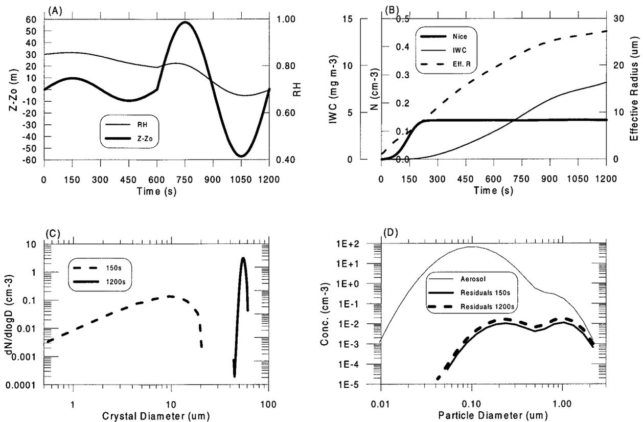
FIG. 3. Simulation results for case 3. (a) Air parcel trajectory with two different wave amplitude; (b) time histories of ice crystal number concentration, ice water content, and crystal effective radius; (c) model-produced ice crystal size distributions at 150 (dashed line) and 1200 s (solid line); and (d) the corresponding residual aerosol size distributions (thick lines) and initial aerosol spectrum (thin solid line).
