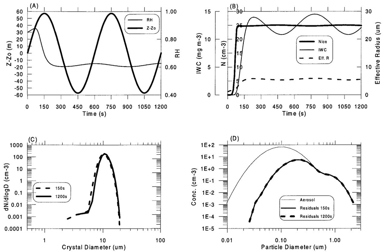
FIG. 2. Simulation results for case 2. (a) Air parcel trajectory with twice the amplitude as in the base case; (b) time histories of ice crystal number concentration, ice water content, and crystal effective radius; (c) model-produced ice crystal size distributions at 150 and 1200 s; and (d) the corresponding residual aerosol size distributions at 150 s and 1200 s (thick lines), and initial aerosol spectrum (thin solid line).
