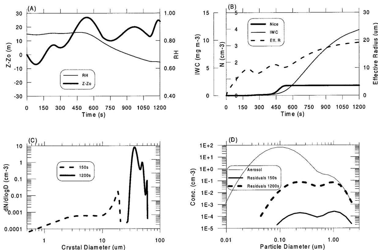
FIG. 5. Simulation results for case 5. (a) Air parcel with a smoothed random walk trajectory; (b) time histories of ice crystal number concentration, ice water content, and crystal effective radius; (c) model-produced ice crystal size distributions at 150 (dashed line) and 1200 s (solid line); and (d) the corresponding residual aerosol size distributions (thick lines) and initial aerosol spectrum (thin solid line).
