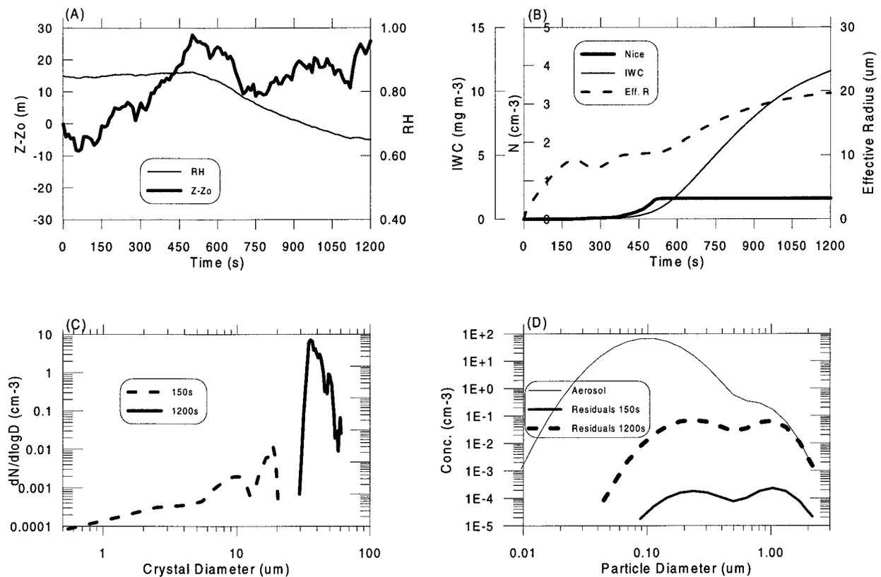
FIG. 4. Simulation results for case 4. (a) Air parcel random walk trajectory, (b) time histories of ice crystal number concentration, ice water content, and crystal effective radius; (c) model-produced ice crystal size distributions at 150 (dashed line) and 1200 s (solid line); and (d) the corresponding residual aerosol size distributions (thick lines) and initial aerosol spectrum (thin solid line).
