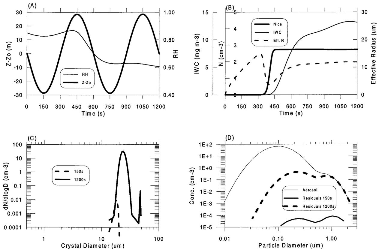
FIG. 6. Simulation results for case 6. (a) Air parcel starting with a position having wave phase  $\varphi = \pi$ , (b) time histories of ice crystal number concentration, ice water content, and crystal effective radius; (c) model-produced ice crystal size distributions at 150 (dashed line) and 1200 s (solid line); and (d) the corresponding residual aerosol size distributions (thick lines) and initial aerosol spectrum (thin solid line).
