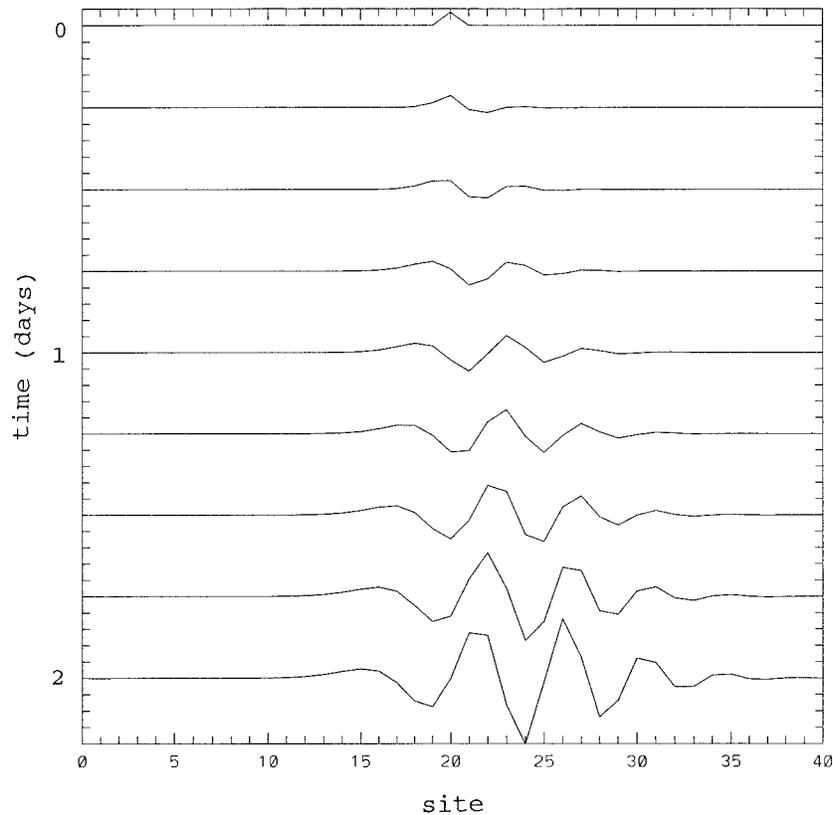
FIG. 1. Longitudinal profiles of  $X_j$  at 6-h intervals, as determined by Eq. (1) with  $N = 40$  and  $F = 8.0$ , when initially  $X_{20} = F + 0.008$  and  $X_j = F$  when  $j \neq 20$ . On horizontal portion of each curve,  $X_j = F$ . Interval between successive short marks at left and right is 0.01 units.
