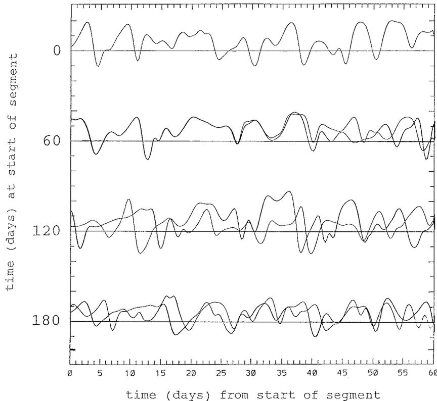
FIG. 4. A time series of  $X_{10}$ , as determined by Eq. (1), originating from the initial state of Fig. 2 and extending for 240 days, displayed as four consecutive 60-day segments. A second time series, produced by adding 0.0001 units to the single variable  $X_{10}$  at the beginning of the second segment, is superposed on the last three segments. Horizontal lines are zero lines. Interval between short marks at left and right is 5.0 units.
