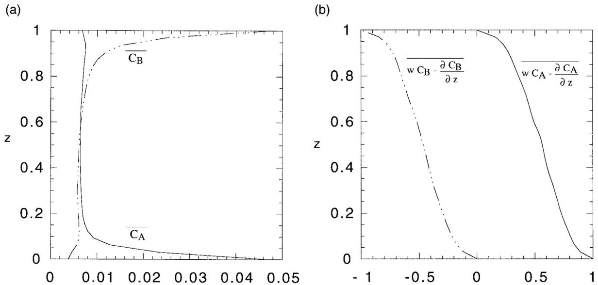
FIG. 3. Vertical profiles ( $Da_d = 4.6 \times 10^4$ ) of (a) the dimensionless horizontally averaged concentration of chemical species and (b) the dimensionless total vertical flux of the chemical species.
