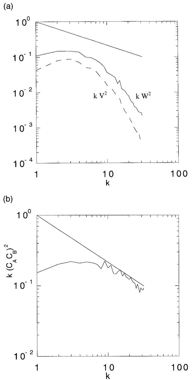
FIG. 2. (a) One-dimensional power spectra of horizontal ( $v$ ) and vertical velocity fluctuations ( $w$ ) and (b) 1D spectrum of covariance between both chemical species (simulation 4). Spectra have been averaged in space and time.
