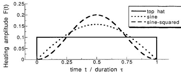
FIG. 1. Nondimensional heating amplitude,  $F(t)$ , as a function of time for the three heating sequences of finite duration. The duration of each sequence is  $\tau$  and the integrated heating is the same for each heating sequence. The solid curve is for the top hat heating, the dashed curve is for the sine-squared heating, and the dotted curve is for the sine heating.
