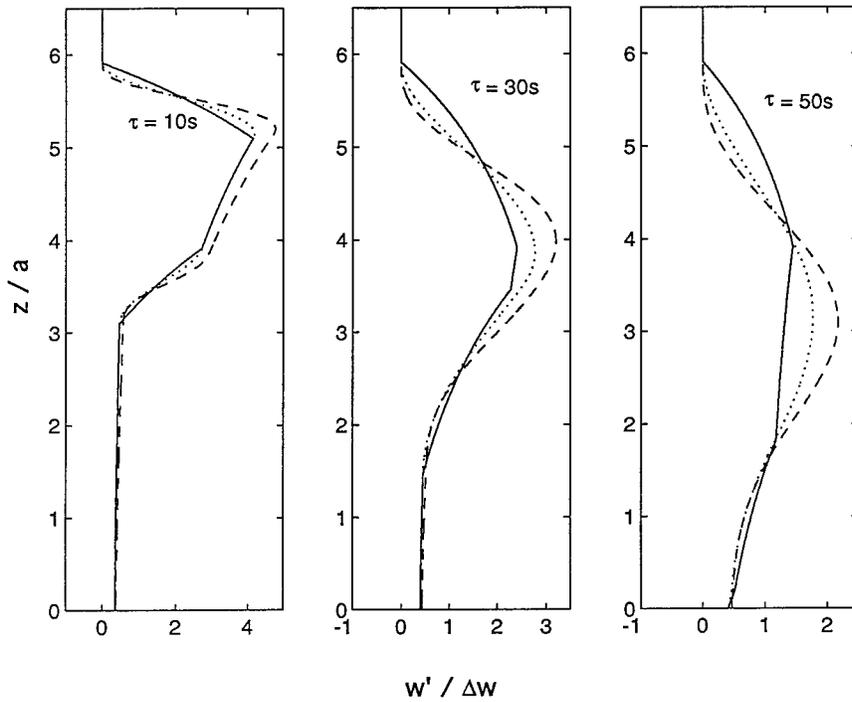
FIG. 5. Vertical velocity fields at  $t = 60$  s as a function of height for the three heatings of finite duration for  $\tau = 10, 30,$  and  $50$  s. The solid curve is for the top hat heating, the dashed curve is for the sine-squared heating, and the dotted curve is for the sine heating.
