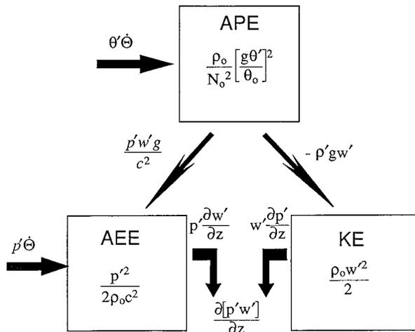
FIG. 7. Schematic diagram of the Eulerian energetics. The relationship between available elastic (AEE), available potential (APE), and kinetic energy (KE) are shown. The direction of the arrows indicates the direction of positive energy transfer.
