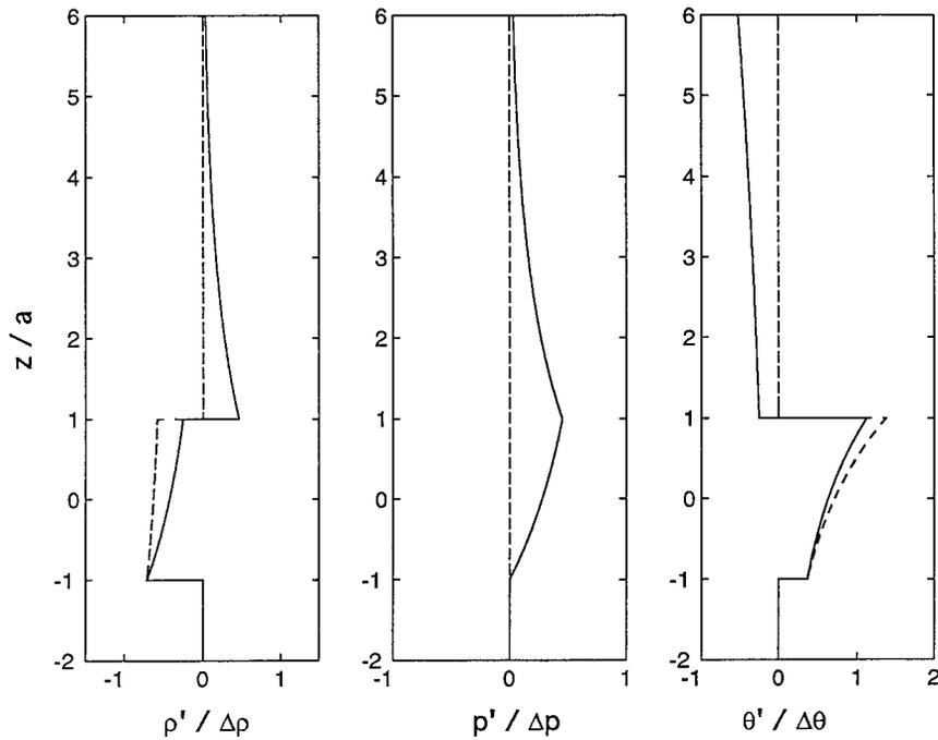
FIG. 6. Final density, pressure, and potential temperature perturbations as a function of height. The solid curves are the Eulerian variables, the dashed curves the Lagrangian variables.
