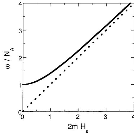
FIG. 2. The dispersion relation for the acoustic-gravity waves (solid curve) produced in the adjustment. The dashed curve corresponds to the pure acoustic case of zero gravity.
