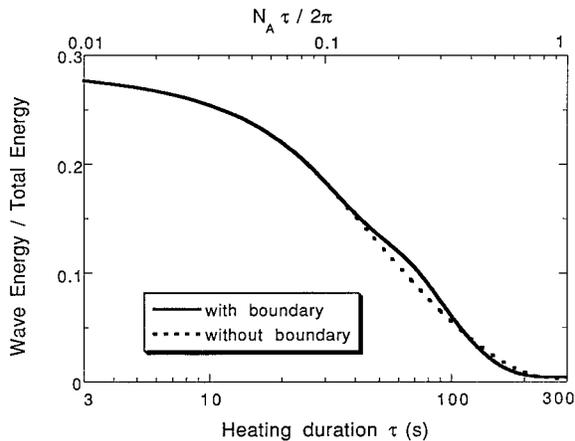
FIG. 10. Wave energy generation as a function of duration for the top hat case with and without a lower boundary at  $z = -2a$ . The wave energy is normalized by the total energy generated.
