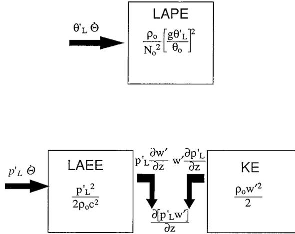
FIG. 8. Schematic representation of the Lagrangian energetics. The Lagrangian available (LAPE), Lagrangian elastic (LAEE), and kinetic energy (KE) are shown. The direction of the arrows indicates the direction of positive energy transfer.
