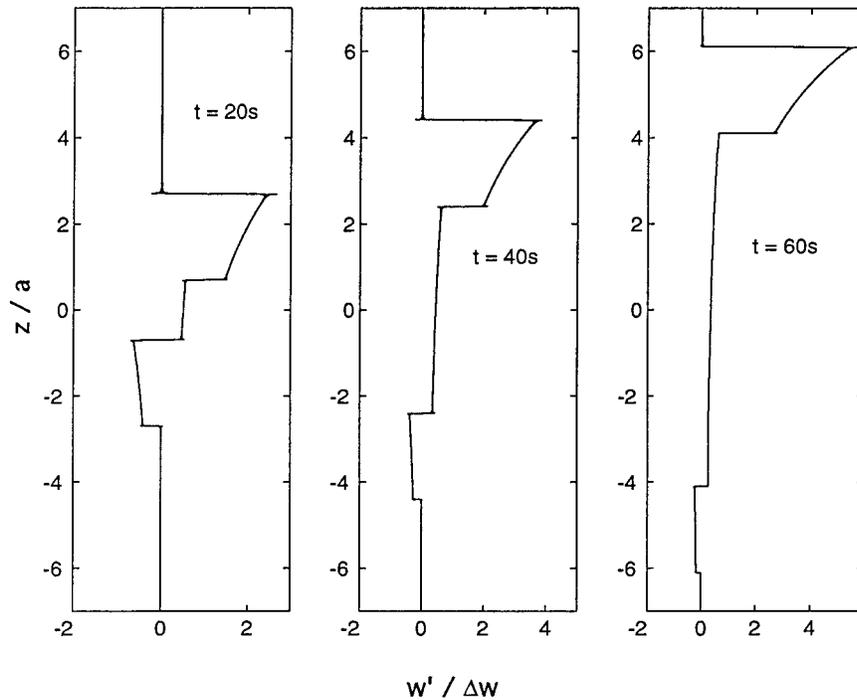
FIG. 3. Vertical velocity fields as a function of height for the case of instantaneous heating at the times  $t = 20, 40,$  and  $60$  s after the heating.
