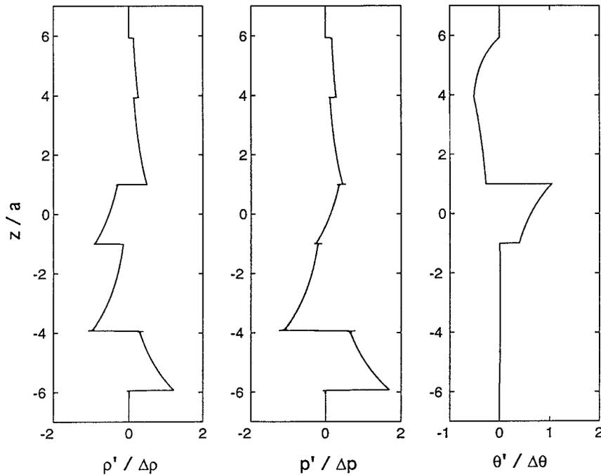
FIG. 4. Density, pressure, and potential temperature fields as a function of height for the instantaneous heating at  $t = 60$  s.
