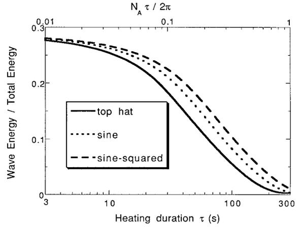
FIG. 9. Wave energy generation as a function of the heating duration  $\tau$  for the three heating sequences. The wave energy is normalized by the total energy generated.
