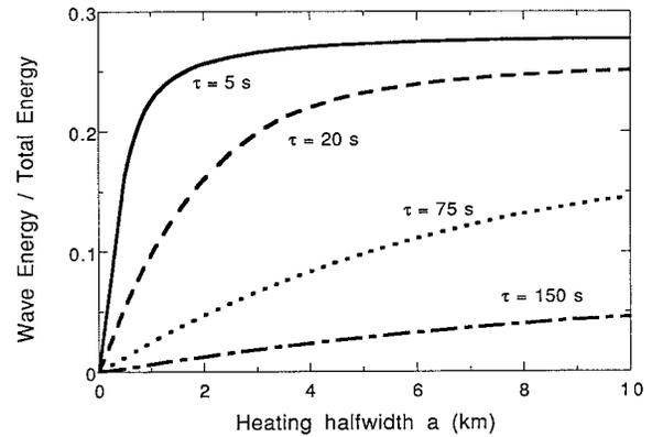
FIG. 11. Wave energy generation as a function of the heating half-width  $a$  for the top hat case for four different values of the heating duration  $\tau = 5, 20, 75,$  and  $150$  s. The wave energy is normalized by the total energy generated.
