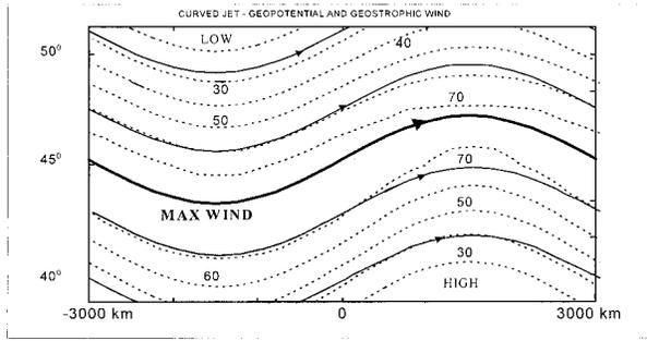
FIG. 10. Geopotential height (solid) and geostrophic wind speed of a curved jet in the steady state calculated from Eqs. (17) and (3). Isotachs (dashed) are drawn in units of  $m\ s^{-1}$  with a  $10\ m\ s^{-1}$  interval. Axes are as in Fig. 3.
