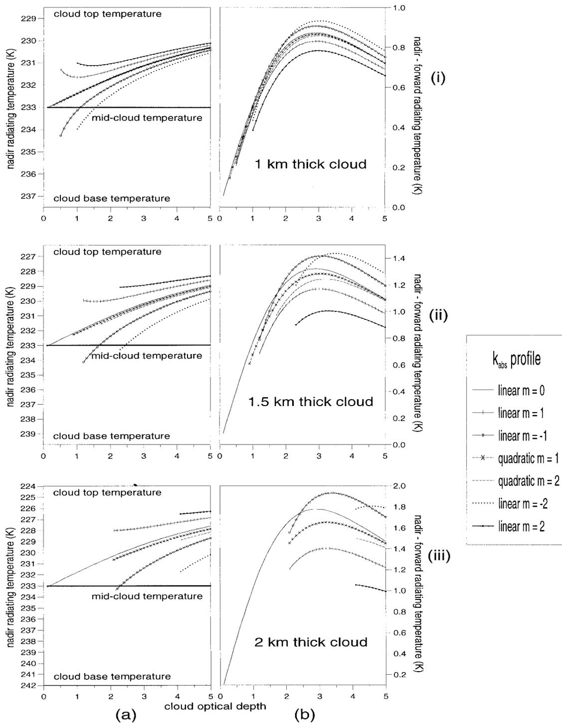
FIG. 6. (a) (left) Nadir-radiating temperature and (b) (right) nadir-minus forward cloud-radiating temperature; as a function of cloud optical depth for (i) 1.0-, (ii) 1.5-, and (iii) 2.0-km thick vertically inhomogeneous clouds with temperature lapse rates of  $9 \text{ K km}^{-1}$  and different absorption coefficient profiles.
