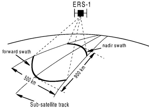
FIG. 1. Viewing arrangement of the ATSR instrument on the ERS-1 satellite.
