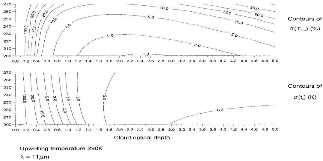
FIG. 2. Contours of uncertainty in the retrieved quantities as a function of cloud temperature for upwelling temperatures of 290 K, 0.5% uncertainty on forward and nadir upwelling and exitant radiances at a wavelength of 11 μm. (upper) Uncertainty in the retrieved cloud optical depth as a percentage of the true cloud optical depth; (lower) uncertainty in retrieved temperature (K).
