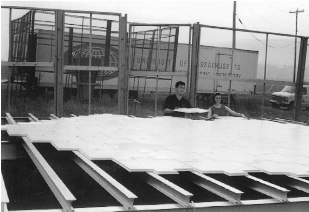
FIG. 1. A photo of the TEP system in Rock Springs, PA. The foreground of the photo shows the receiver array encased within a clutter fence. Visible behind the array is the transmitter horn and the operations trailer.
