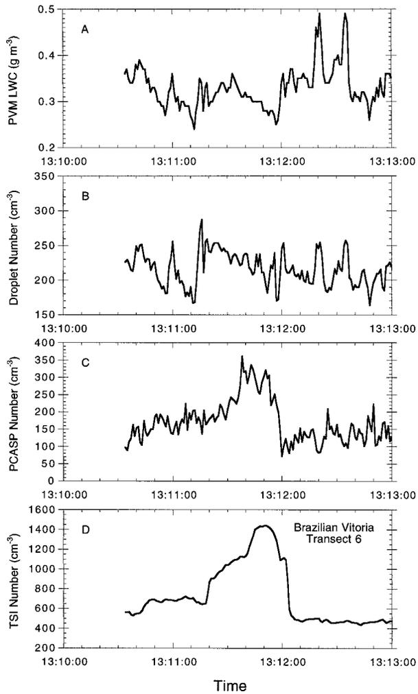
FIG. 5. Time series for transect 6, 8.5 km the *Brazilian Vitoria*. Track age was approximately 3 h. Measurements were made aboard the UW C-131A. (a) Liquid water content from PVM-100A; (b) droplet number concentration from PMS FSSP-100X; (c) accumulation-mode aerosol number concentration from PCASP 100-X; (d) aerosol number concentration from TSI 3760 condensation particle counter.
