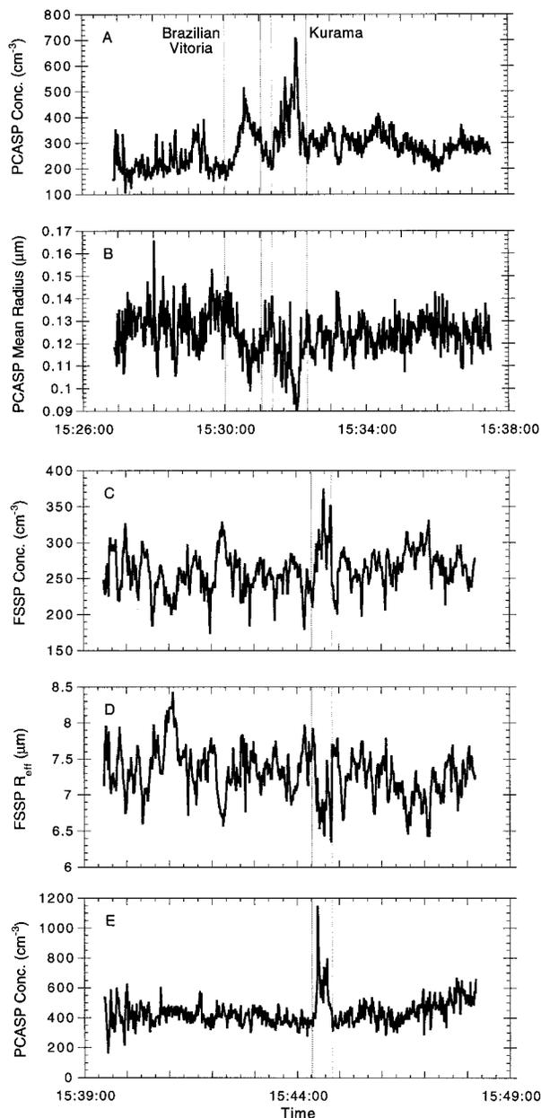
FIG. 13. Time series for two crossings of the *Kurama* ship track. (a) and (b) are for a transect near the point at which the two tracks crossed. (c)–(e) are for a second transect of the *Kurama* track. The shaded areas indicate plume encounters. Instruments: PCASP-100 (a), (b), and (e); FSSP-100 (c) and (d). Measurements made from the MRF C-130.
