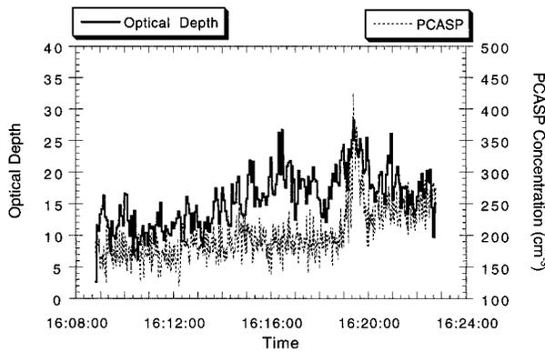
FIG. 15. Cloud optical depth and accumulation-mode concentration time series across the *Kurama* track. Instruments: PCASP-100; optical depth derived from MCR nadir reflectance measurements at 1.25 and 2.26  $\mu\text{m}$ . Measurements from the MRF C-130.
