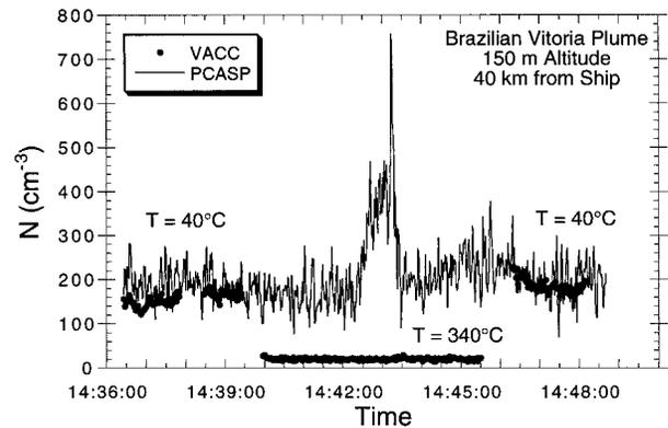
FIG. 12. Time series of aerosol at (near) ambient temperature, 40°C and 340°C, for a below-cloud transect of the *Brazilian Vitoria* plume. Measurements made with the UMIST VACC system on the MRF C-130.
