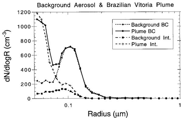
FIG. 11. Comparison of aerosol size distributions (below cloud and interstitial) measured at 40°C for the background and *Brazilian Vitoria* plume. Measurements made with the UMIST VACC system on the MRF C-130.
