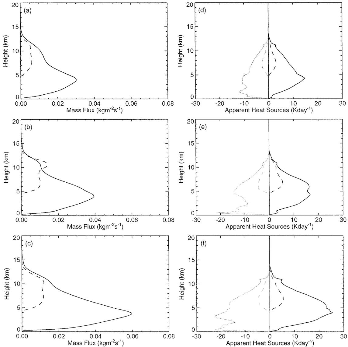
FIG. 4. (a) Nine-hour means of mass flux for MCS2. The solid line represents the convective core mass flux and the dashed line the mesoscale updraft mass flux. (b) as (a) but for MCS3. (c) as (a) but for MCS5. (d) Nine-hour means of  $Q_1$  (black lines) and  $-Q_2$  (gray lines) for MCS2. Again the convective updraft is a solid line and the mesoscale updraft the dashed line. (e) as (d) but for MCS3. (f) as (d) but for MCS5.
