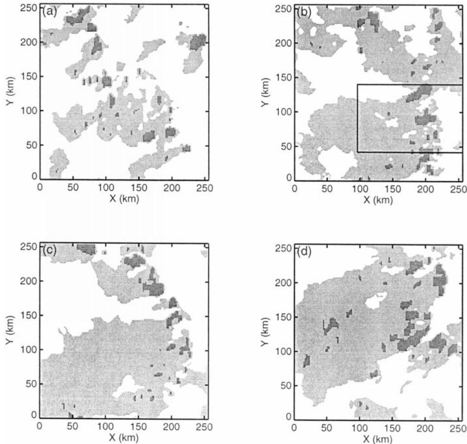
FIG. 2. Horizontal structure of the simulated MCSs at (a) 36 h, (b) 63 h, (c) 69 h, and (d) 111 h. Convective columns are shaded dark gray and stratiform columns light gray. A definition of the column classification used is given in the text. The rectangle in (b) represents the area used in the vertical cross section in Fig. 3.
