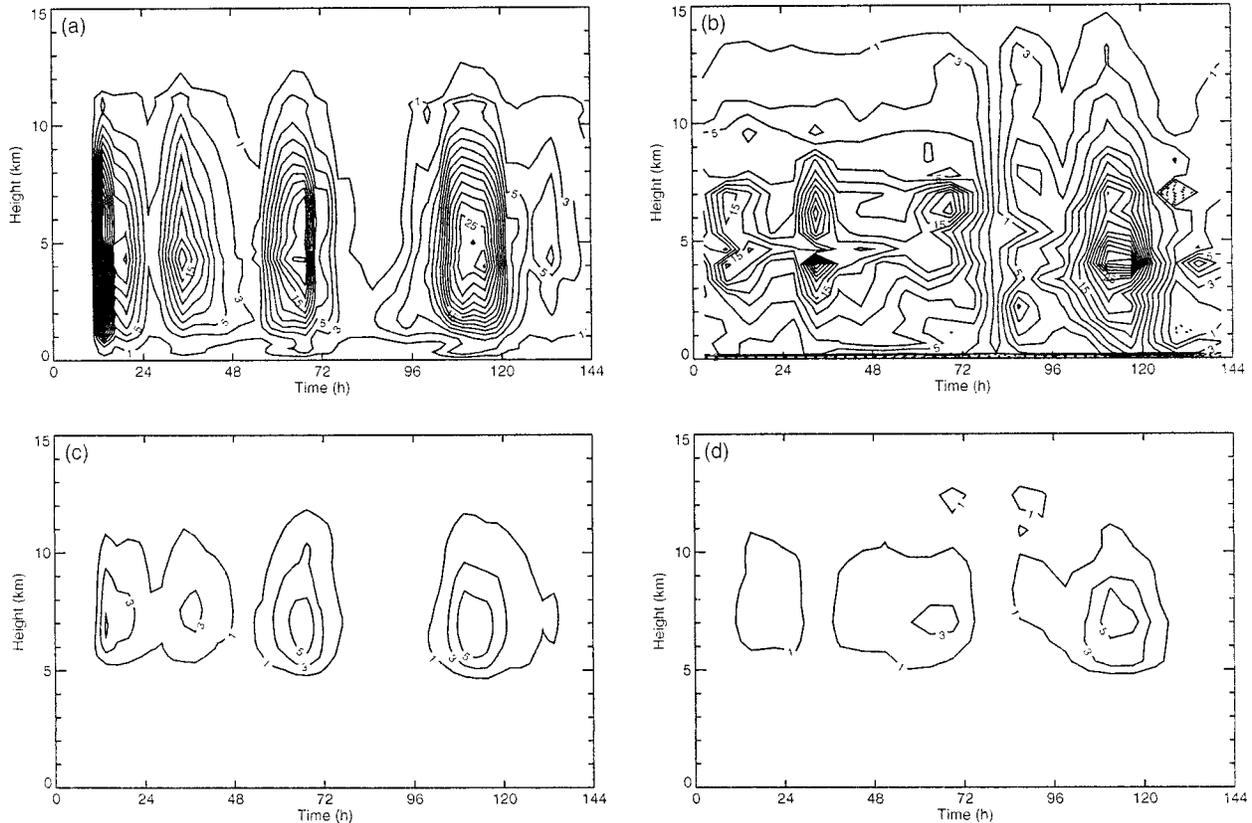
FIG. 10. Convective updraft heating rates for (a) CRM and (b) SCM experiments, and (c) mesoscale updraft heating rates for CRM and (d) SCM. Contour interval is  $2 \text{ K day}^{-1}$  with the first contour at  $1 \text{ K day}^{-1}$ .
