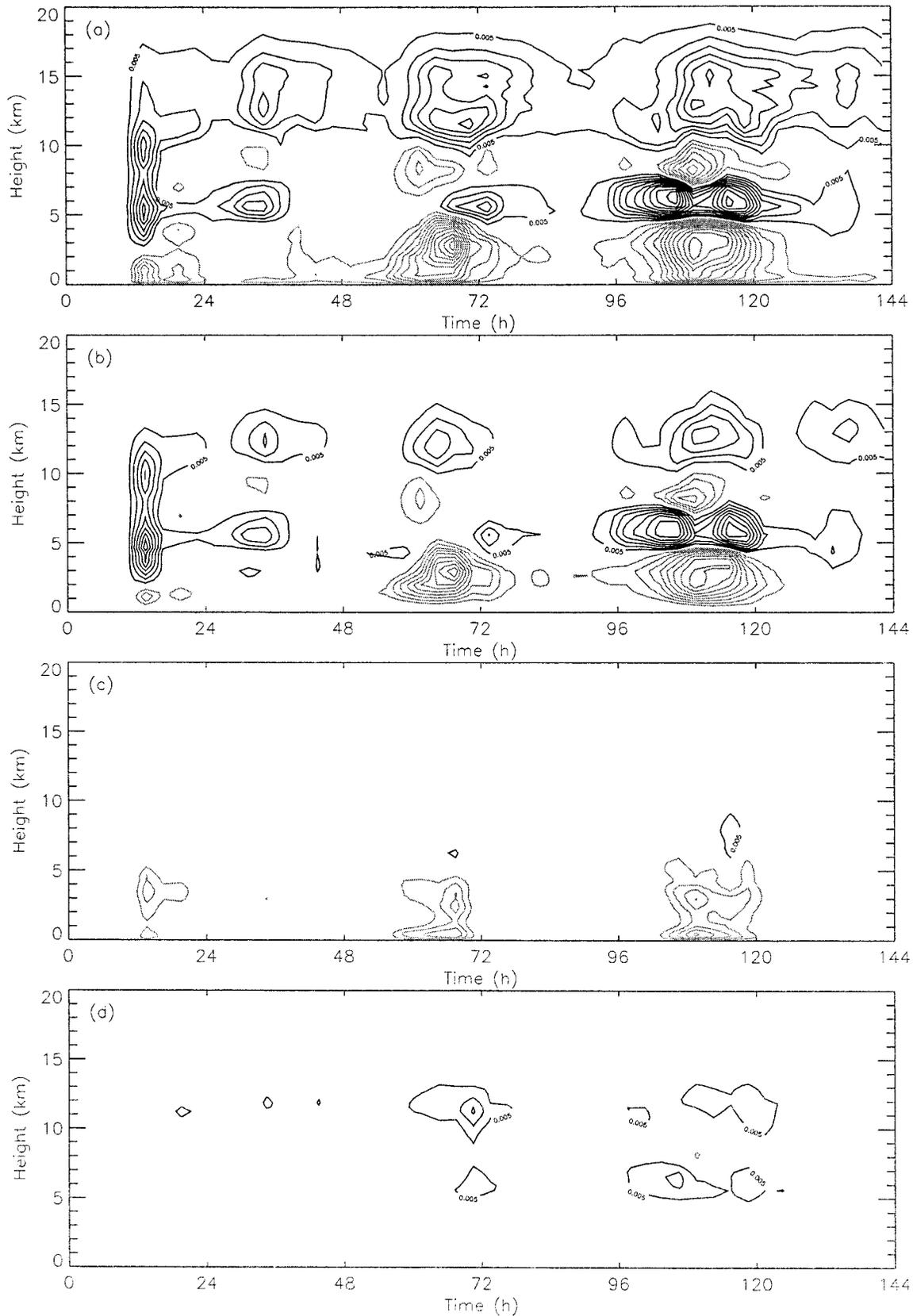
FIG. 7. Zonal momentum flux diagnosed from the CRM simulation for (a) all points, (b) convective updrafts, (c) precipitating downdrafts, and (d) mesoscale updrafts. Contour interval is  $0.01 \text{ m}^2 \text{ s}^{-2}$ , first contour at  $0.005 \text{ m}^2 \text{ s}^{-2}$ , and negative values are shown in gray.
