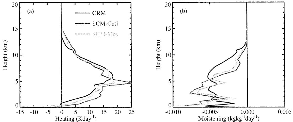
FIG. 12. Comparison of (a) apparent convective heat source and (b) apparent convective moisture source, averaged over day 5 for the CRM (black line), the SCM without a mesoscale updraft and downdraft parameterization (SCM-Cntl, medium gray line), and the SCM with a mesoscale updraft and downdraft parameterization (SCM-Mes, light gray line).
