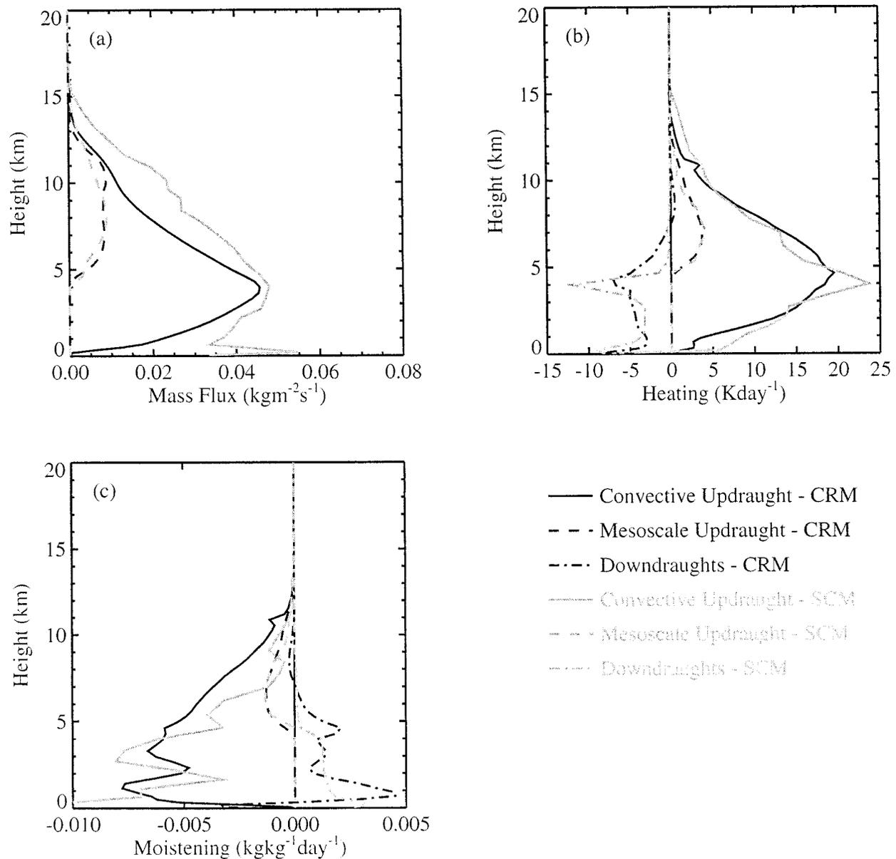
FIG. 11. Comparison of (a) mass fluxes, (b) heating rates, and (c) moistening rates between the CRM and SCM simulations averaged over day 5 of the simulation. Convective updrafts are shown by solid lines, mesoscale updrafts by dashed lines, and downdrafts by dash-dot lines. Results from the CRM are shown as black lines and results from the SCM are shown as gray lines.
