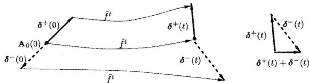
FIG. 2. Defining  $\Theta$ : equal and opposite perturbations at  $t = 0$ ,  $\boldsymbol{\delta}^\pm(0)$ , evolve so as to be no longer symmetric at time  $t$ . The error in assuming linear dynamics,  $\|\boldsymbol{\delta}^+(t) + \boldsymbol{\delta}^-(t)\|$ , is scaled by the average magnitude of the evolved perturbations to give the relative nonlinearity  $\Theta$ .
